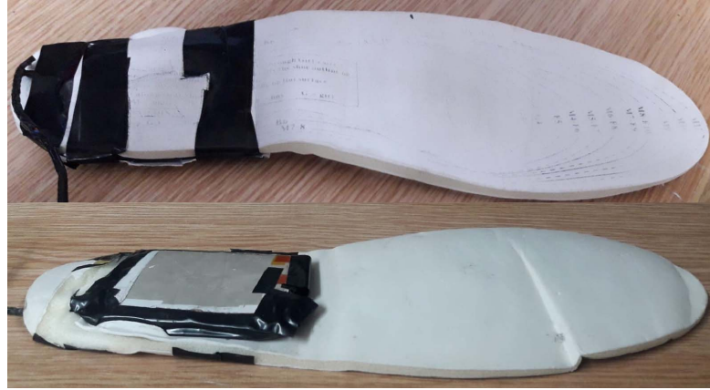
Figure 5.8: 50-layer polypropylene ferroelectret energy harvester mounted in a shoe insole.
