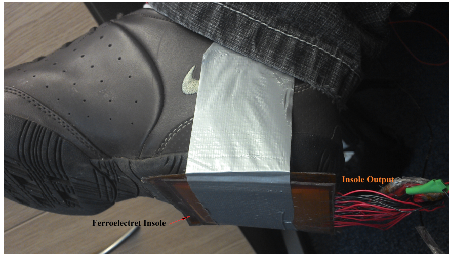
Figure 3.2: Sole Method. The insole is placed in the sole of the shoe.
