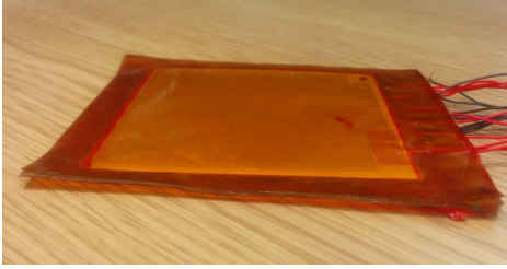
Fig. 3. 30-layer ferroelectret insole used in our design.
