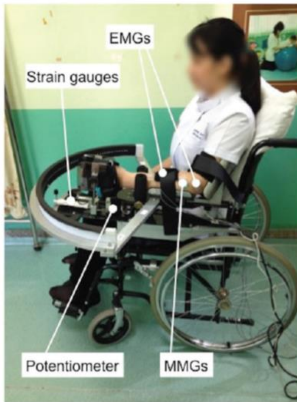
Figure 2. Participant set up in the wrist rig showing force sensors, angle sensors, sEMG attached to the forearm flexors and location of MMG sensors on the forearm flexors.
