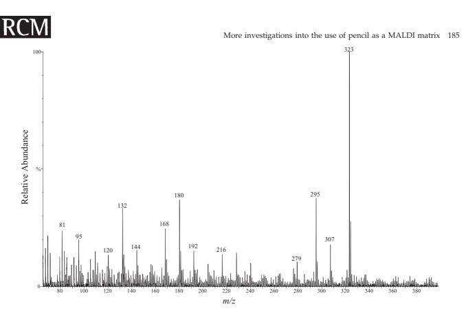
**Figure 3.** MALDI-TOF mass spectrum of PL matrix showing the presence of hexadecanoic acid  $[M+Na]^+ m/z$  279 and  $[M+K]^+ m/z$  295 with octadecanoic acid  $[M+Na]^+ m/z$  307 and  $[M+K]^+ m/z$  323.
