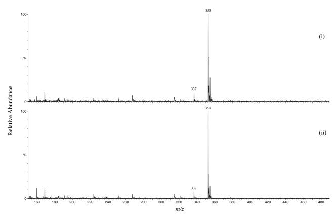
**Figure 8.** MALDI-TOF mass spectra of ranitidine using (i) 2B PL matrix on a new target plate and (ii) 2B PL matrix on a used and cleaned target plate where m/z 337 =  $[M+Na]^+$  and m/z 353 =  $[M+K]^+$ .
