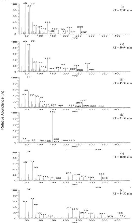
**Figure 5.** El mass spectra of selected peaks from gas chromatograms: (i) hexadecanoic acid CAS#57-10-3, (ii) octadecanoic acid CAS#57-11-4, (iii) decyl oleate CAS#3687-46-5, (iv) dibutyl phthalate CAS#84-74-2, (v) tetracosane CAS#646-31-1, and (vi) tetratetracontane CAS#7098-22-8.
