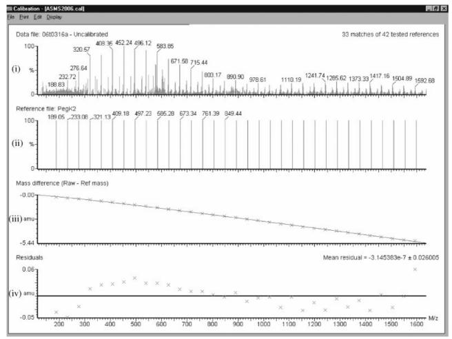
Figure 9. Mass calibration from a Cali-Pen showing (i) data file, (ii) reference file, (iii) linearity of calibration, and (iv) residual errors in mass calibration.
