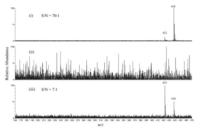
**Figure 1.** (i) MALDI-TOF mass spectrum of colchizine using 2B PL matrix at 50% coarse, 50% fine laser power; (ii) LDI-TOF mass spectrum of colchizine at 50% coarse, 50% fine laser power; and (iii) LDI-TOF mass spectrum of colchizine at 100% coarse, 100% fine laser power, where m/z 422 =  $[M+Na]^+$  and m/z 438 =  $[M+K]^+$ .
