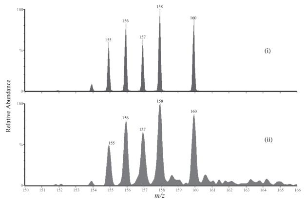
Figure 6. Theoretical isotope pattern (i) and MALDI-TOF mass spectrum (ii) of gadolinium ion from gadolinium nitrate using 2B PL matrix.
