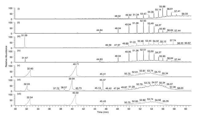
**Figure 4.** GC total ion current chromatograms of DCM solvent extracts of pencil lead from different makes and grades of pencil: (i) Dixon<sup>®</sup> 2B, (ii) Woolworths 2B, (iii) Niceday CGG 100 HB, (iv) Niceday CGG 75 HB, (v) Staedtler 2B, (vi) Steadtler Mars 2B, and (vii) Staedtler Mars 6B.
