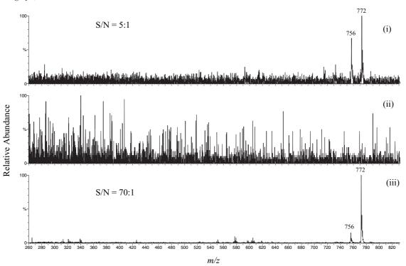
**Figure 7.** MALDI-TOF mass spectra of erythromycin with (i) insufficient PL matrix, e.g. HB pencil; (ii) excessive PL matrix, e.g. 6B pencil; and (iii) routine amount of PL matrix as deposited with a 2B pencil where m/z 756 =  $[M+Na]^+$  and m/z 772 =  $[M+K]^+$ .
