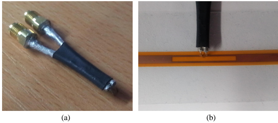
Figure 7. Photographs of the coaxial jig used to measure the antenna's impedance (left) and the coaxial tips landing (right).
