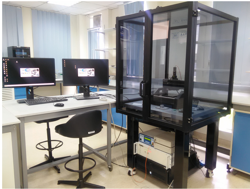
Figure 3.5: Laser Profiler using TaiCaan TM machine
