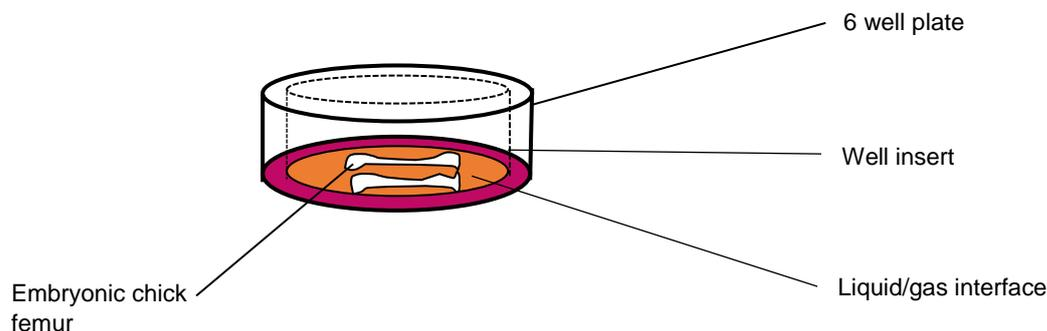
**Figure 6.1 Schematic diagram of the *ex vivo* organotypic culture system of embryonic chick femora**
