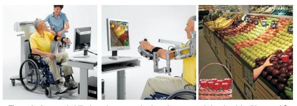
**Figure 2.** Armeo rehabilitation robot, arm orthosis and screen, and virtual activity (Hocoma AG 2009)
