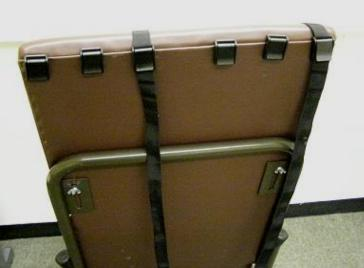
Figure 20 Chair with harness and adjustable positions for harness.
