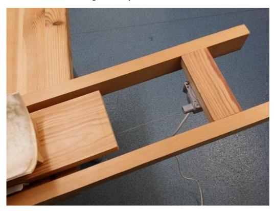
Figure 18 Linear potentiometer.
