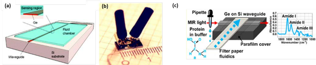
Figure 6 a) Scheme of the Ge waveguide spectroscopy sensor for liquids: a) a microfluidic chamber can be bonded onto the substrate, b) Image of the Ge waveguide bonded to the microfluidic channel: the microfluidic channel is 1 mm wide, 7mm long, and 50 \mu\text{m} deep, c) Germanium on Silicon waveguides showing BSA protein detection using filter paper as the microfluidic channel. Reprinted with permission from [56] Copyright (2018) Royal Society of Chemistry and [59] Copyright (2019) American Chemical Society respectively.
