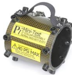
Figure 5.8. 5 cm Mini-Test collar assembly for Plant Integrity Ltd (Plant integrity ltd.,2012).
