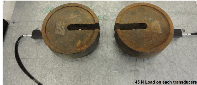
Figure 5.9. Experimental setup of two transducers and two modules on plate. 45N load was applied on each module due to the clamping force.
