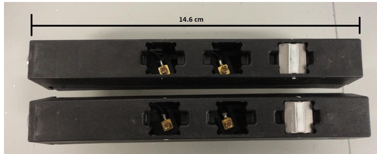
Figure 5.2. Two modules with 6 places for transducers when two transducers are already placed. When modules are placed on a pipe, transducers motion is in shear format.
