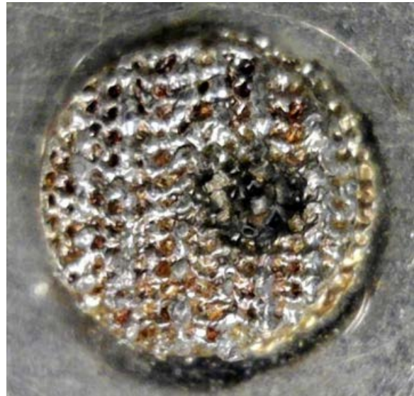
Fig. 4 Ag/Ni contact processed by electron beam processing, to create a highly structure surface.
