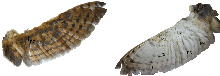
Figure 3: Upper and lower side of Wing 3 of the barn owl samples, showing the positions at which air flow resistance was measured.
