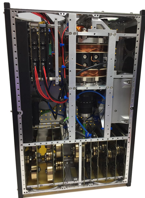
Fig. 11 Final integrated CASPA system, including all subsystems, the printed circuit boards (PCBs) at the bottom of the picture were made to be mass representative of the avionics for vibration testing. The payload can be seen in the top 4U of the photograph
