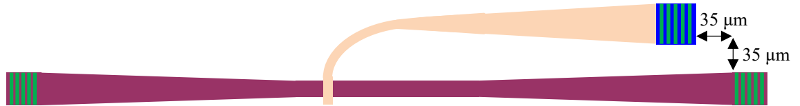
Figure 6.5 Schematic structure of the second-level waveguide placed above the first level waveguide.
