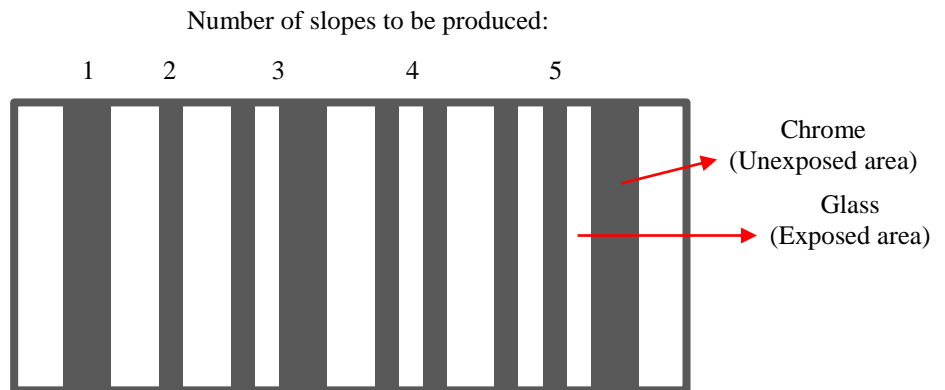
Figure 5.1 Schematic diagram of the optical mask design illustrating the multiple bars used to define the slope platform.
