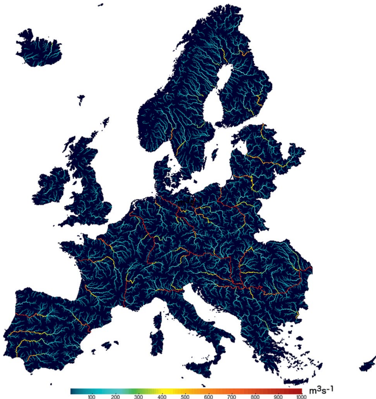
FIG. 2. Simulated mean daily streamflow from 1950 to 2011 for the EDgE domain at 5-km spatial resolution. Simulated daily runoff was obtained with the mHM model forced with downscaled E-OBS forcing data. River routing was carried out with the mRM algorithm.
