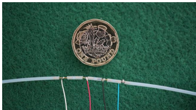
Figure 3.14 Prototype contacting four-electrode array. The separation between the electrodes is visible. One pound coin for scale.
