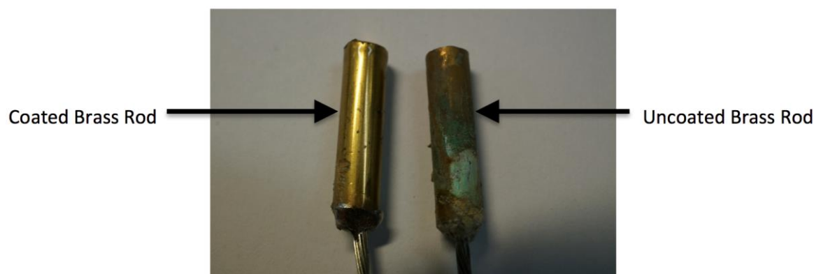
Figure 3.9 Incralac-coated (left) and non-coated (right) brass rods following exposure to seawater over a period of several months.
