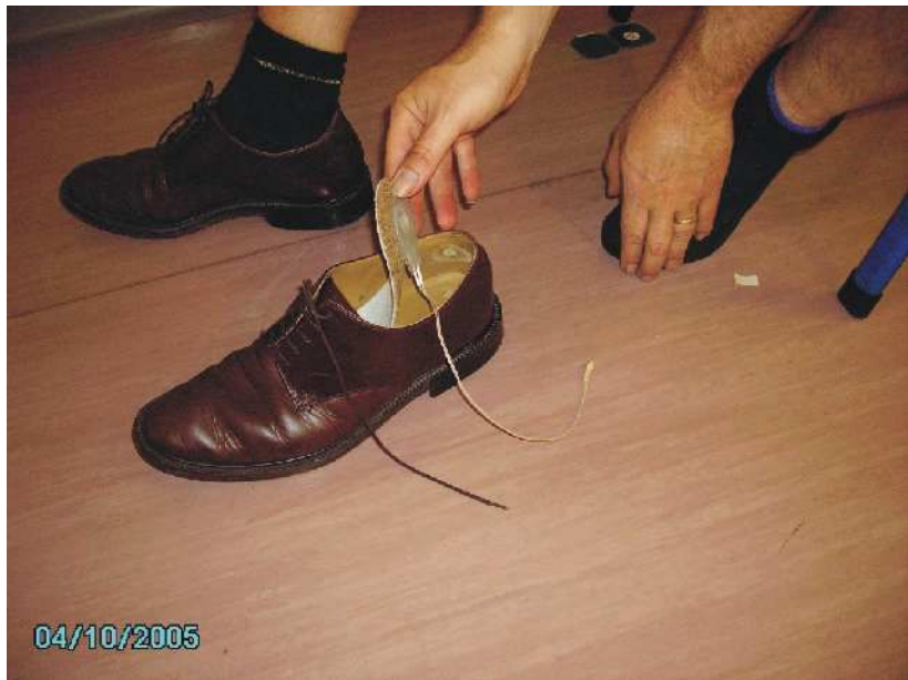
Figure 3. The device is controlled using a pressure sensitive footswitch placed on the underside of an insole.
