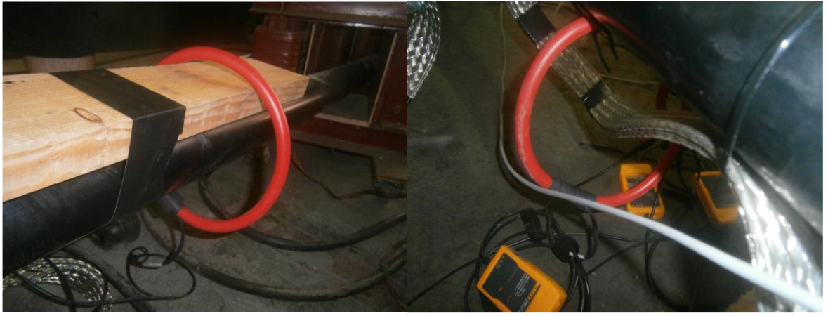
FIGURE 5.9: Measurements of Conductor (on the Left) and Sheath (on the Right) Currents via Rogowski Coils Placed as Centrally as Possible.
