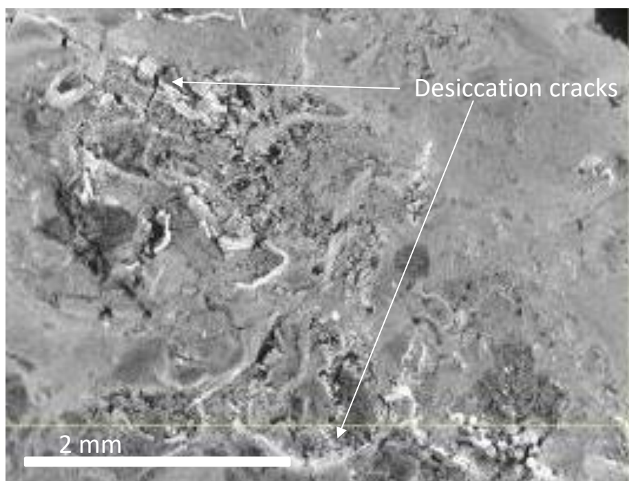
Figure 134: CT scan image of desiccation cracks preserved on the cut surface of 050RD/P3 core sample
