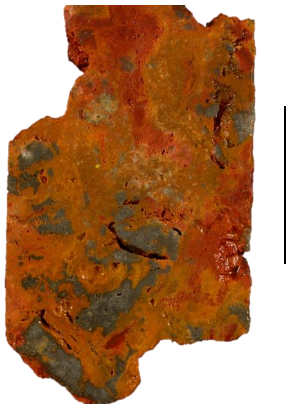
Figure 43: 050RD/P11, example of Unit C. Material recovered is dominated by yellow brown iron oxides with patches of darker red iron oxides. A characteristic feature of this unit is patches of grey silica with disseminated sulphide within. Scale bar = 5cm.
