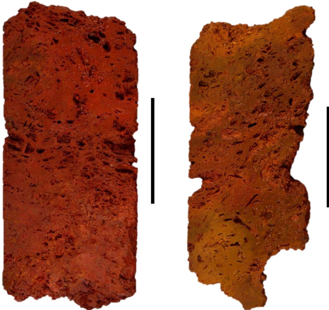
Figure 48: 073RD/Piece 6 (left) and 073RD/Piece 14 (right) shows the variation in colour composition of Unit B material at the MIR mound. Scale bars = 5cm.
