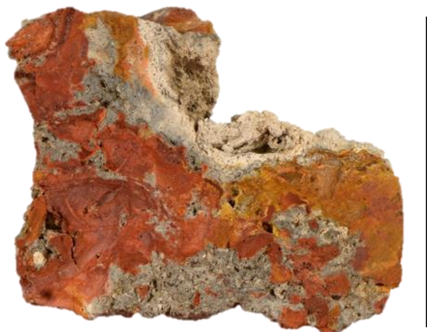
Figure 46: Unit C sample with characteristic grey silica patches, material is silicified red and orange brown iron oxides/oxyhydroxides. Scale bar = 5cm.
