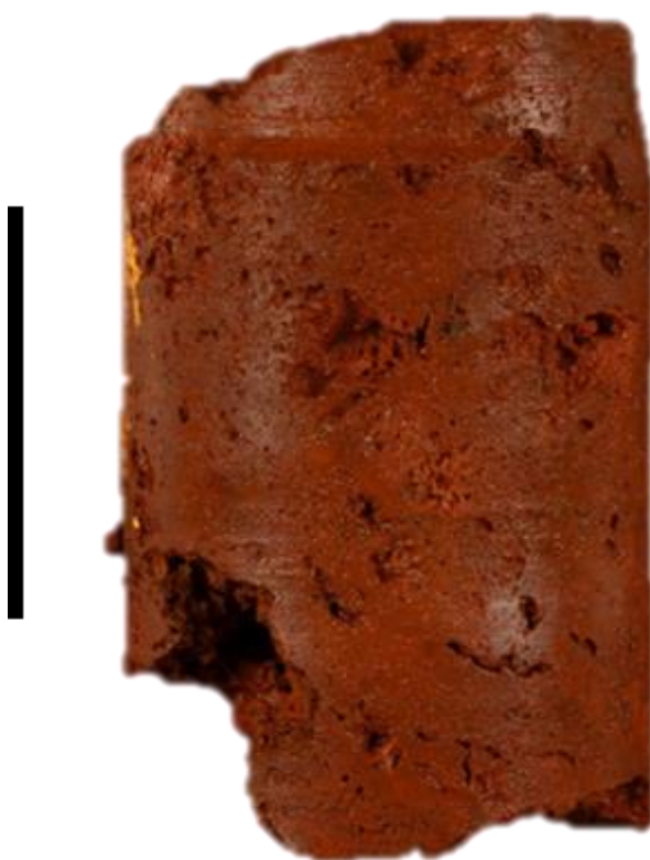
Figure 42: 031RD/107/CC, example of sample from Unit B. Material is dominated by red iron oxide and is notably harder than Unit A. Pore spaces visible at cm scale. Scale bar = 5cm.
