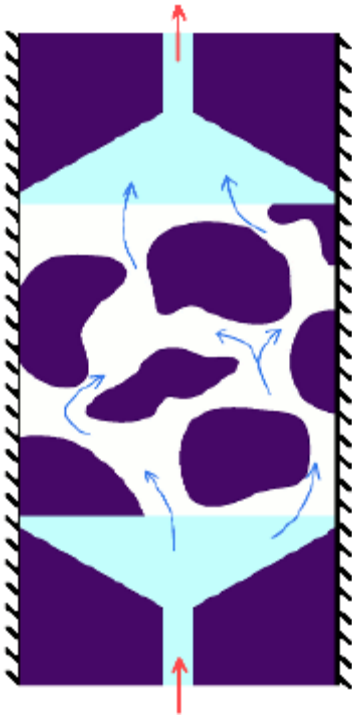
Figure 141: 2D cross section of the experimental setup for absolute permeability simulation in the Avizo software
