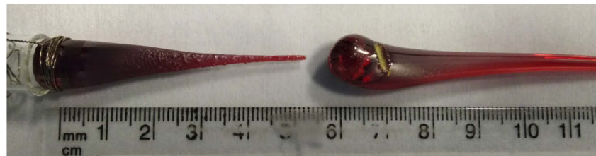
Fig. 14. First and last part of the extruded rod after fibre drawing, where the neck presents some surface crystallization due to the time consumed in the whole process.
