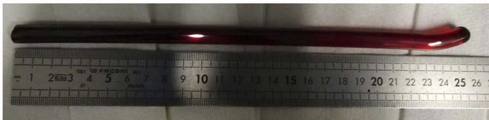
Fig. 1. Extruded structured preform based on GLS-Se glasses.
