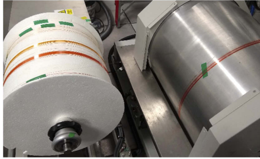
Fig. 19. GLS-Se structured optical fibre being transferred from the drum to a bobbin.
