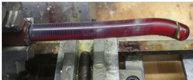
Fig. 5. Extruded rod during polishing.
