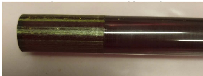
Fig. 6. Surface scratched rod, showing the benefits of polishing.
