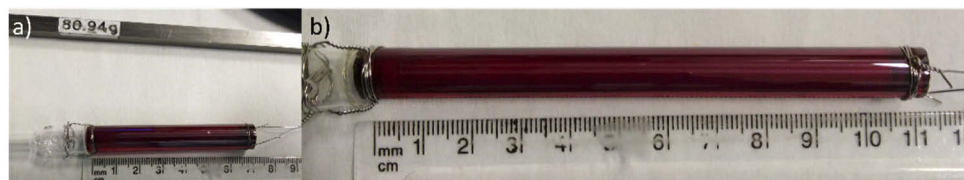
Fig. 9. Examples of extruded and polished rods where a) is attached to the silica holder and the 80 g weight, and b) has a length of 11 cm and is ready to be set on the furnace. Surface quality is clearly seen.
