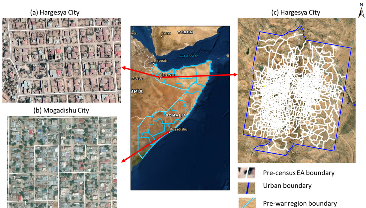
Fig. 6 Outlines of semi-automated urban EAs in different locations over Hargeysa and Mogadishu in Somalia. a, b The automated urban EA boundaries are matching well with ground roads and they are nested within urban strata (c).
