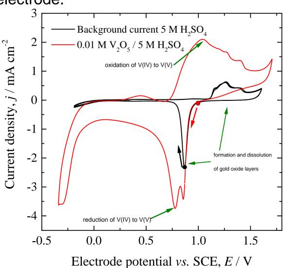
Cyclic voltammograms for the VO<sub>2</sub>+/VO<sup>2+</sup> redox couple at the **gold** electrode.
