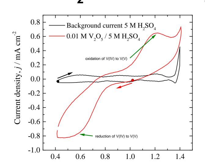
Electrode potential vs. SCE, E / VCyclic voltammograms for the VO<sub>2</sub>+/VO<sup>2+</sup> redox couple at the **DSA 1 (49.66% IrO<sub>2</sub>, 49.66% SnO<sub>2</sub>,** 0.68% Sb<sub>2</sub>O<sub>5</sub>) electrode.
