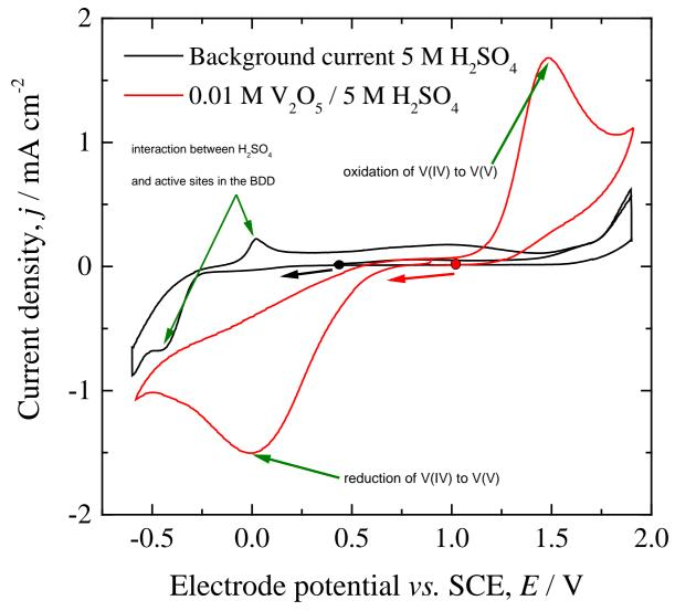
Cyclic voltammograms for the VO<sub>2</sub>+/VO<sup>2+</sup> redox couple at the **boron doped diamond** electrode.
