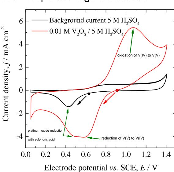
Cyclic voltammograms for the VO<sub>2</sub>+/VO<sup>2+</sup> redox couple at the **platinum** electrode.
