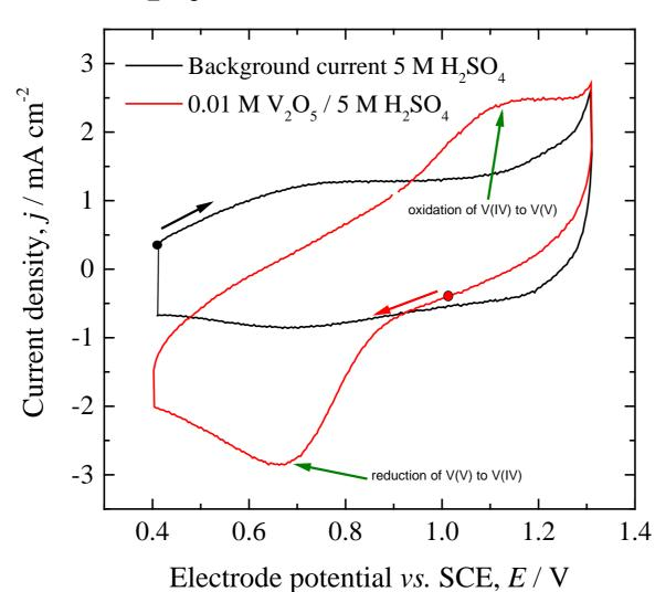
Cyclic voltammograms for the VO<sub>2</sub>+/VO<sup>2+</sup> redox couple at the **DSA 2 (15.4% IrO<sub>2</sub>, 64.6% SnO<sub>2</sub>,**
