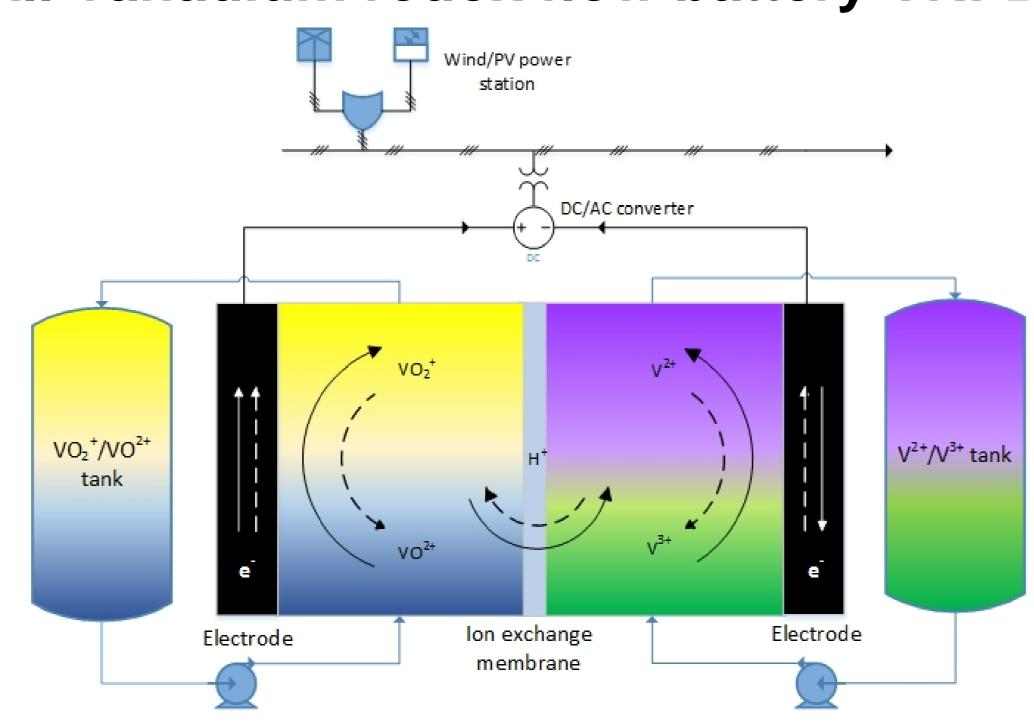
$VO^{2+} + H_2O \stackrel{\text{charge}}{\rightleftharpoons} VO_2^+ + 2H^+ + e^- E^\circ = 1.0 \text{ V vs. SHE}$  $V^{3+} + e^{-} \rightleftharpoons_{\text{discharge}}^{\text{charge}} V^{2+} E^{\circ} = -0.26 \text{ V vs. SHE}$
