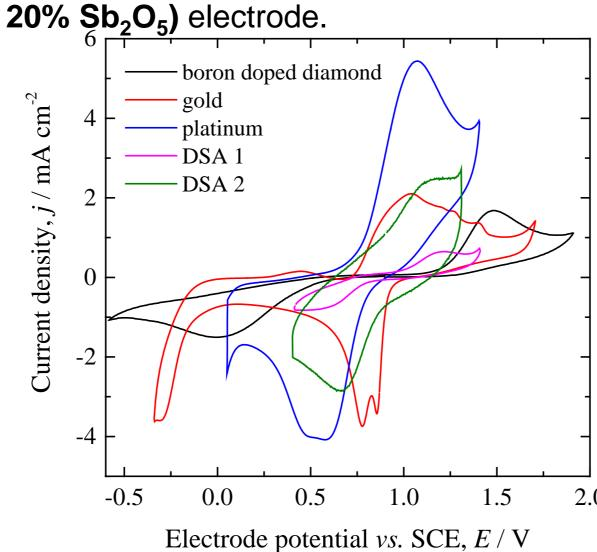
Electrode material CV comparison
