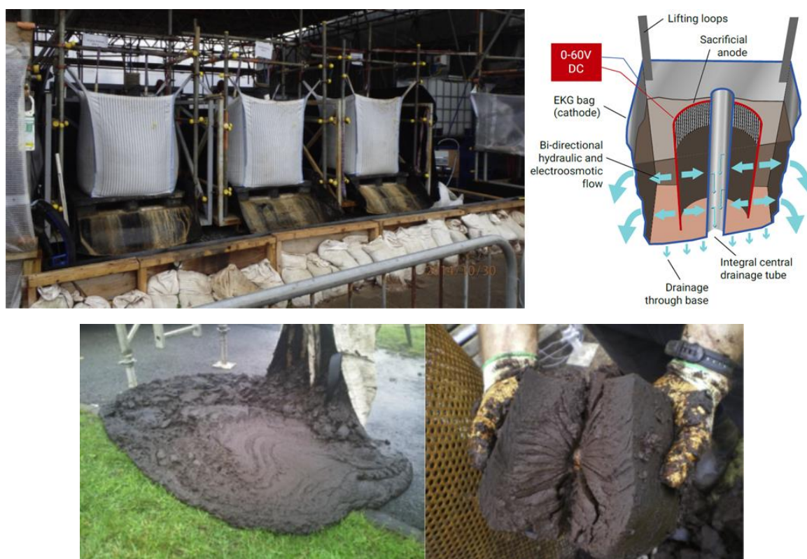
Figure 21 – Top: batch scale processing of contaminated nuclear waste sludges on site; bottom: contaminated sludge before and after processing. Figures adapted from Lamont-Black et al. 144
