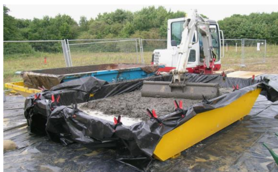
Figure 7 – Left, ex-situ processing of plutonium contaminated waste by Agnew et al. at the Atomic Weapons Establishment (AWE), UK, plus scale and electrode arrangement used on the right. 51
