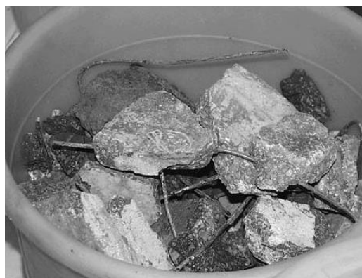
Figure 6 – Examples of the concrete examined by Yurchenko et al. , 48 complete with reinforced steel pins used in construction. X-ray (Rietveld) analysis indicated \alpha -quartz, orthoclase and plagioclase feldspar, calcite and boltwoodite – \text{H}(\text{K},\text{Na})(\text{UO}_2)(\text{SiO}_4) \cdot 1.5(\text{H}_2\text{O}) – phases in the concretes.
