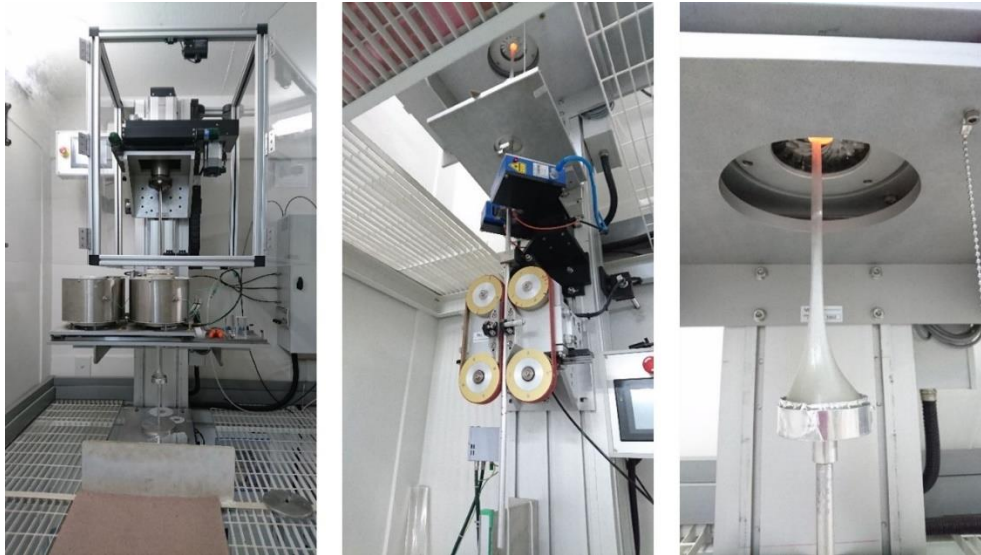
Figure 3.8 The pulling process of the cane.
