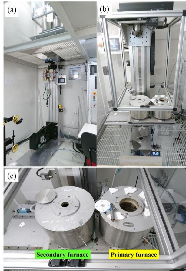
Figure 3.6 (a) The drawing tower, (b) and (c) furnaces used to heat the fibre preform and fibre cane during the drawing process.
