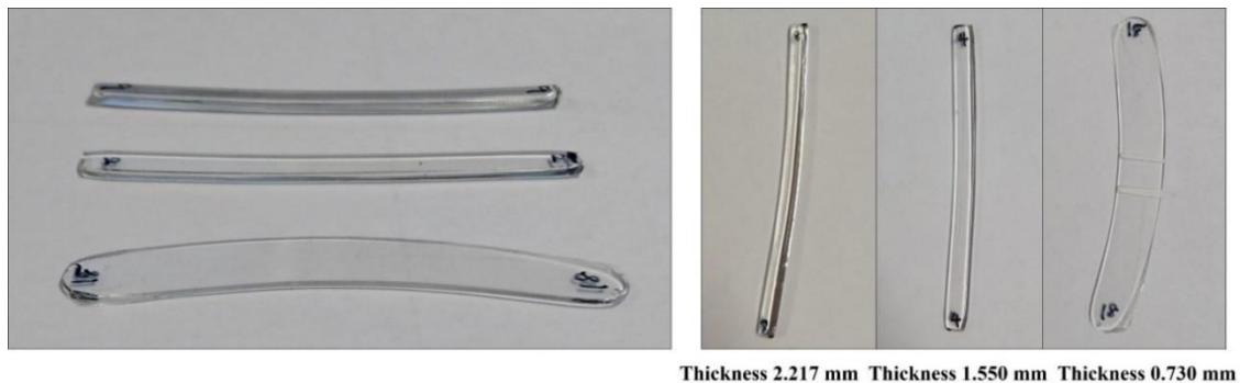
Figure 3.12 Different thickness flat PETG samples for material absorption measurements.
