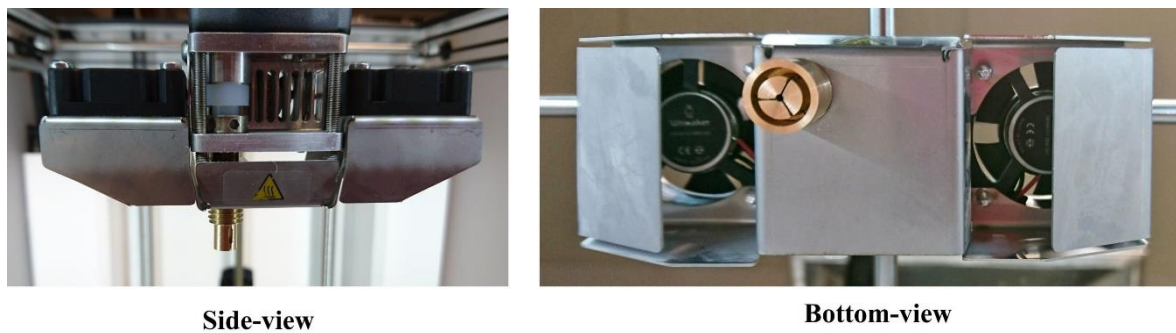
Figure 4.4 Micromachined structured nozzle connected with the heating area of the 3D printer.
