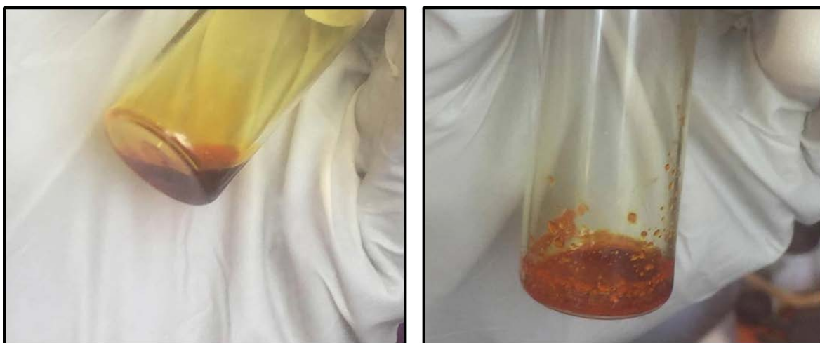
Figure 3.5.4 – Pictures of the saturated polysulfide solution (left) and the precipitate from a supersaturated polysulfide solution (right).
