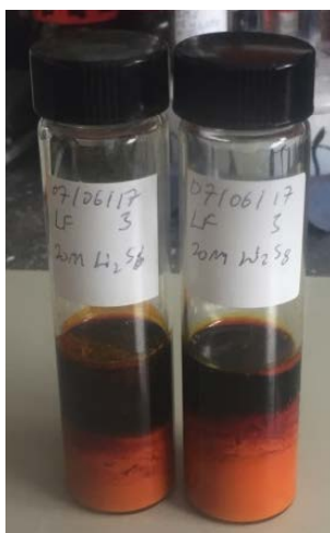
Figure 3.5.3 – “[ S ] _T^{Sol} = 20 M, Li_2S_6 ” (left) and “[ S ] _T^{Sol} = 20 M, Li_2S_8 ” (right) polysulfide blends after heating at 60 °C and stirring for a month then left to cool down to room temperature for 1 week.
