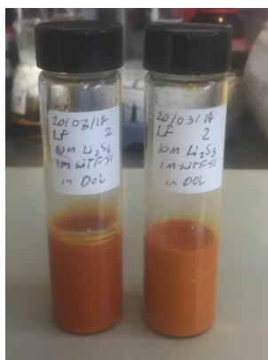
Figure 3.5.2 – “[ S ] _T^{Sol} = 10 M, Li_2S_6 ” (left) and “[ S ] _T^{Sol} = 10 M, Li_2S_8 ” (right) polysulfide blends after heating at 60 °C and stirring for 2 weeks.
