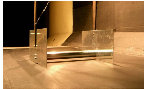
FIG. 2. Model installation in the wind tunnel.
