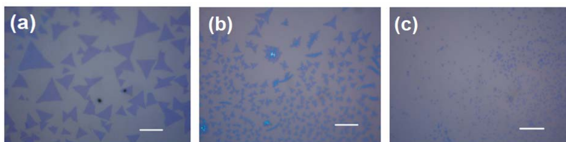
Figure 57 – Optical images of MoS 2 at different locations: the distances from MoO 3 are (a) 3 cm, (b) 5 cm and (c) 7 cm. W_{Sulphur} = 150 mg, T_{Sulphur} = 200 °C, W_{MoO_3} = 15 mg, T_{Substrate} = 700 °C, ramping rate = 10 °C/min, flow rate = 30 sccm. Scale bar is 50 \mu m.
