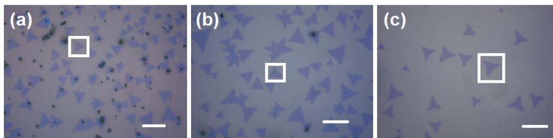
Figure 52 – Optical images of MoS 2 synthesized with different sulfur amounts: (a) 100 mg, (b) 150 mg and (c) 200 mg. The amount of MoO 3 is 15 mg; temperatures of MoO 3 and S are 700 and 200 °C, respectively; ramping rate is 10 °C/min; flow rate is 30 sccm. Scale bar is 50 μm.
