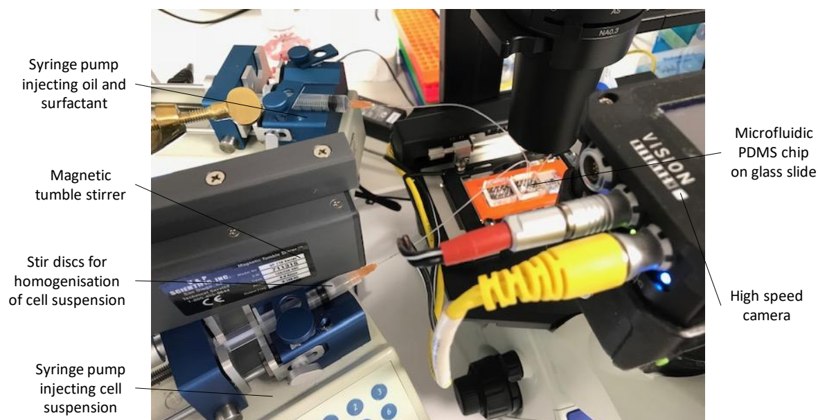
Figure 5.5 Experimental set-up for droplet generation and characterisation of soft lithography chips. Two syringe pumps inject the carrier phase consisting of oil and surfactant and the aqueous phase (i.e. cell suspension), respectively. Cell aggregation in the latter is prevented by continuous stirring of the cell suspension through stir discs that are powered by a magnetic tumble stirrer. The microfluidic device is fitted to the microscope stage using a holder and is connected to the syringes and the collection tube via tubings. Live videos are captured during droplet generation by the high speed camera.
