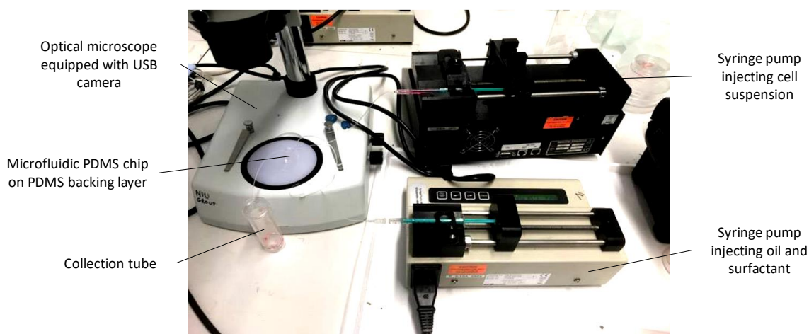
Figure 5.3 Experimental set-up for PDMS chip testing consisting of microscope, chip and tubing, collecting tube, syringes and syringe pumps.
