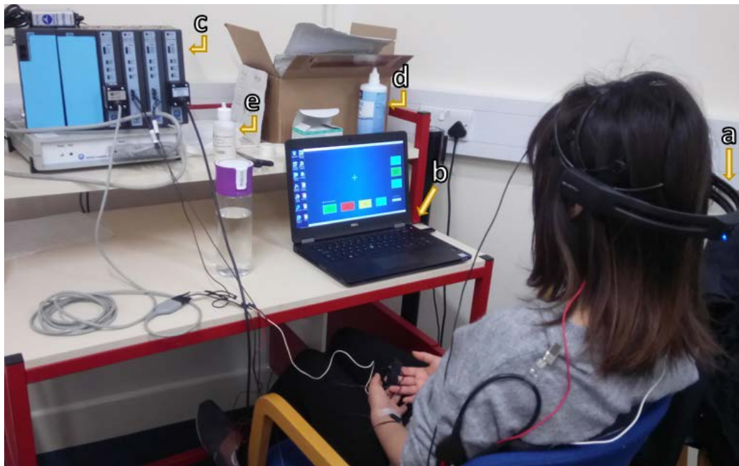
Figure 5.2 Set-up of Emotiv headset and the Biopac MP100
