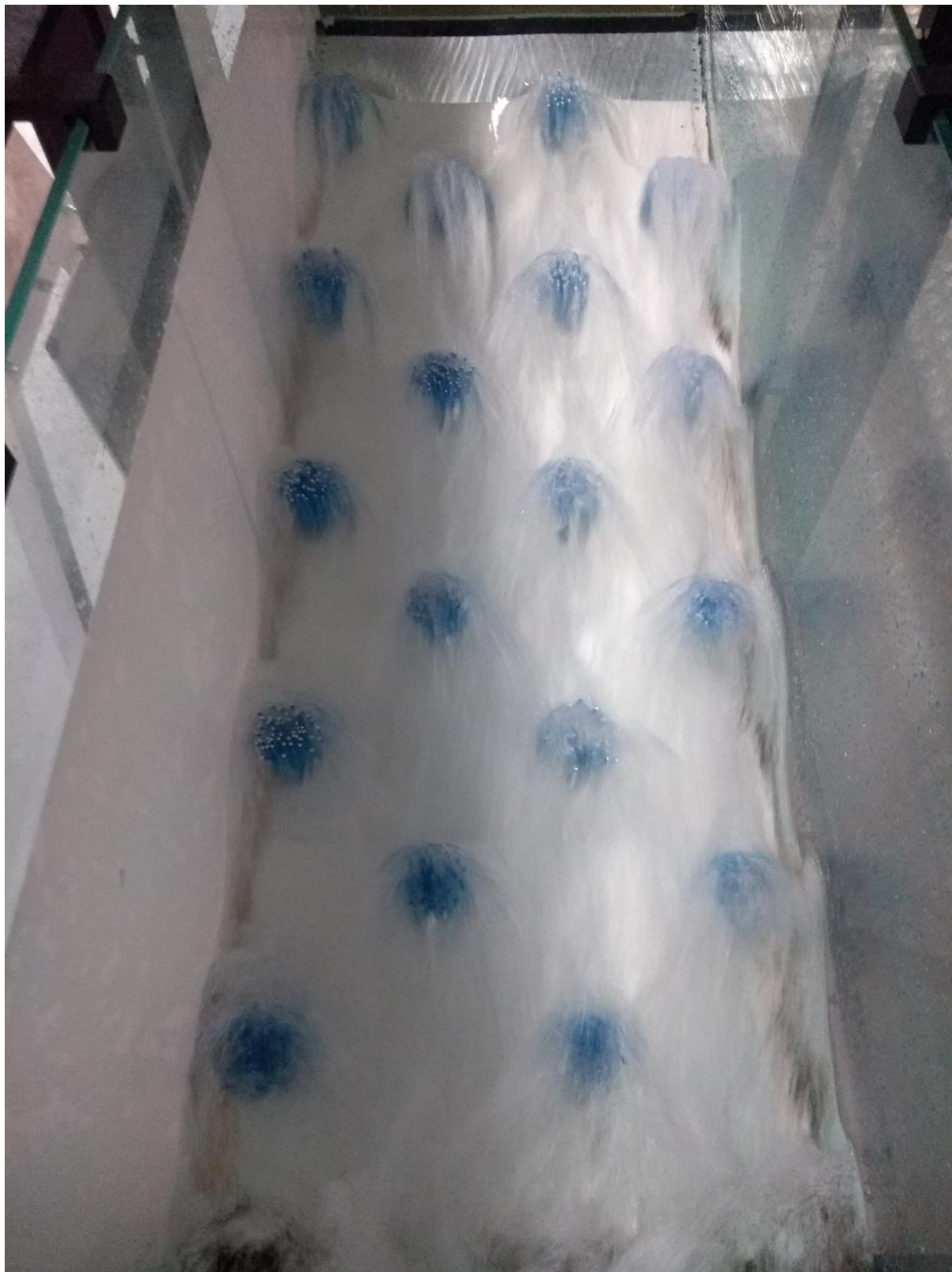
Figure A.6.2 Photograph from above with water running through a staggered array of clusters with 0.15 m diagonal spacing and 0.07 m diameter clusters.
