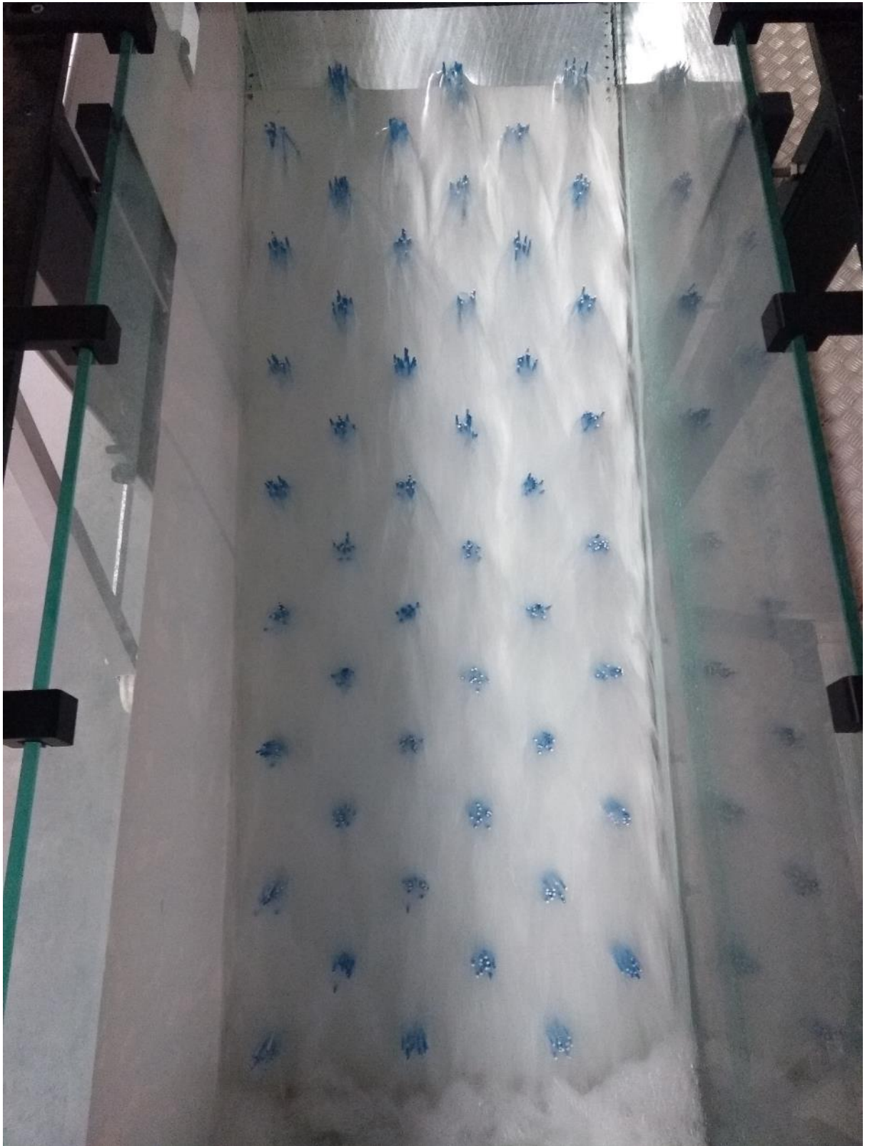
Figure A.6.3 Photograph from above with water running through a staggered array of clusters with 0.1 m diagonal spacing and 0.03 m diameter clusters.
