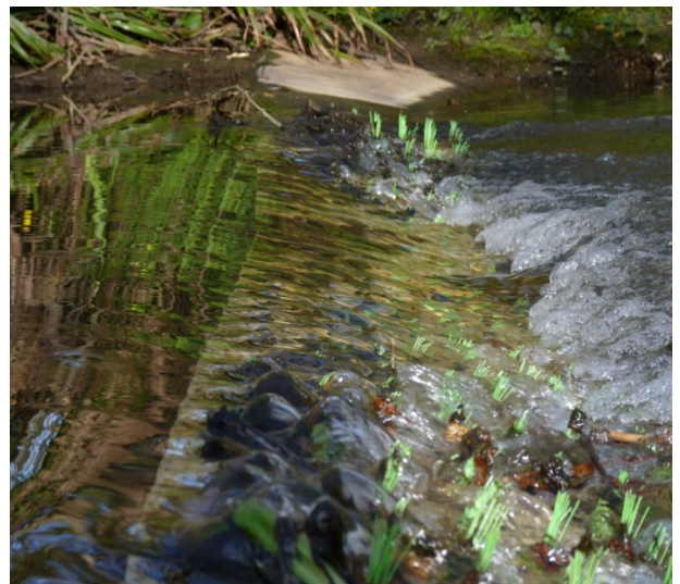
Figure 4.10 Debris accumulation within the bristles over a flat-V weir in (a) laboratory and (b) field conditions.
