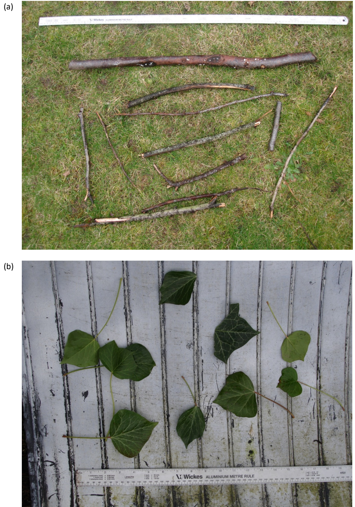
Figure 4.4 A sample of the debris that was tested during debris experiments undertaken in the laboratory showing the representative size and type of debris used during experiments.
