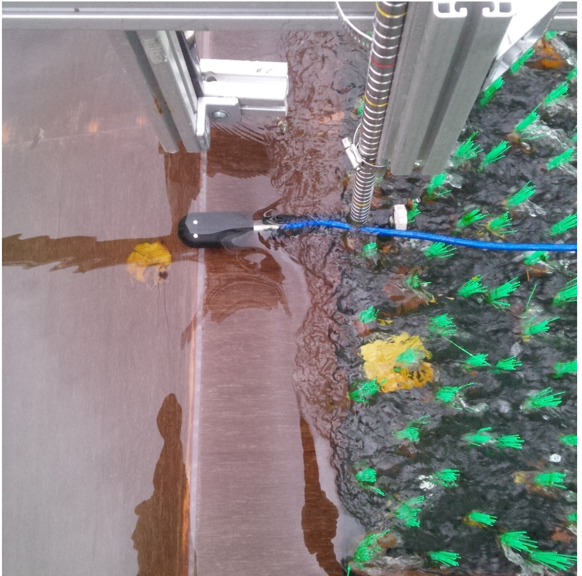
Figure A.1.4 Photograph of the velocimeter used to measure water velocities measuring water velocity at the weir crest upstream of the clusters.
