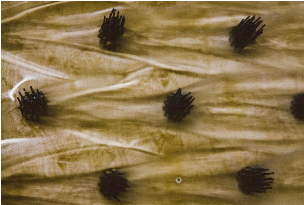
Figure A.7.12 Plan view of a number of unsubmerged CBCs with water flowing from left to right showing the water diverging around the clusters and the wakes created.
