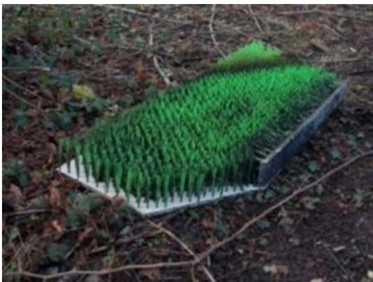
Figure 2.7 A bristle board comprising of conical synthetic bristle clusters fixed onto a plastic board.
