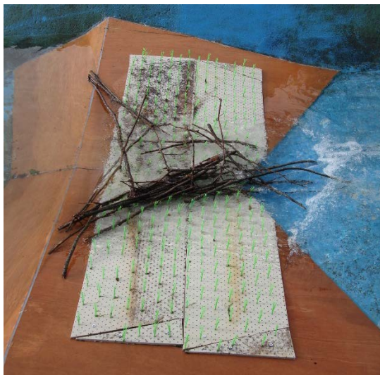
Figure 4.10 Debris accumulation within the bristles over a flat-V weir in (a) laboratory and (b) field conditions.
