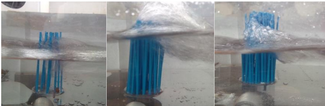
Figure 6.13 Flow around a cylindrical cluster at different levels of submergence.
