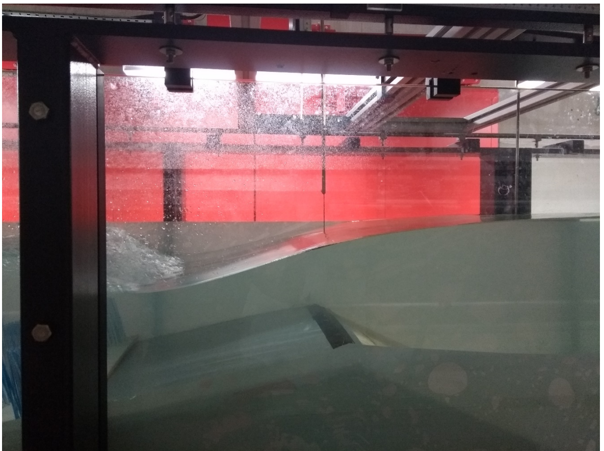
Figure A.4.3 Photograph of the weir crest and water surface profile over the crest when the tailwater level was raised sufficiently that the hydraulic jump formed just prior to the first line of clusters.
