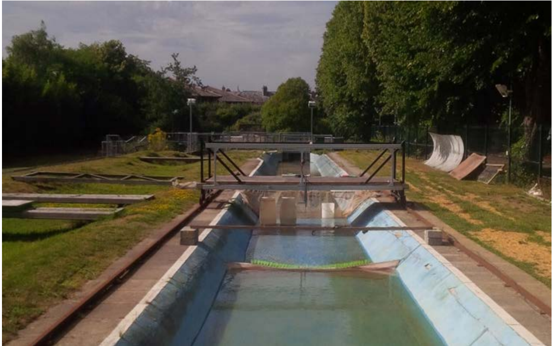
Figure A.1.1 Experimental setup showing the flume with the flat-V weir inserted looking downstream.
