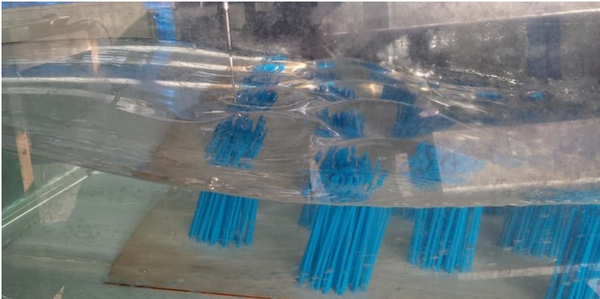
Figure A.7.8 Water surface profile over the 0.07 m diameter CBCs when submerged slightly showing an undulating water surface.
