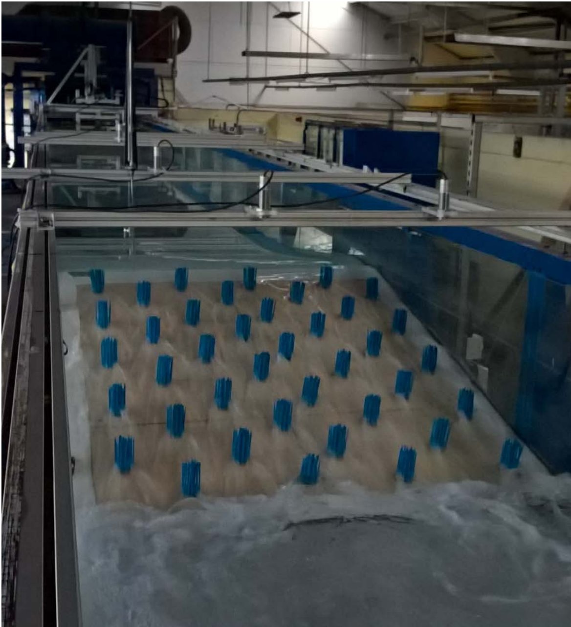
Figure 6.7 Photograph of the experimental setup looking upstream showing the CBCs mounted onto the downstream Crump weir face within the flume with water flowing through the clusters and a hydraulic jump at the weir base.
