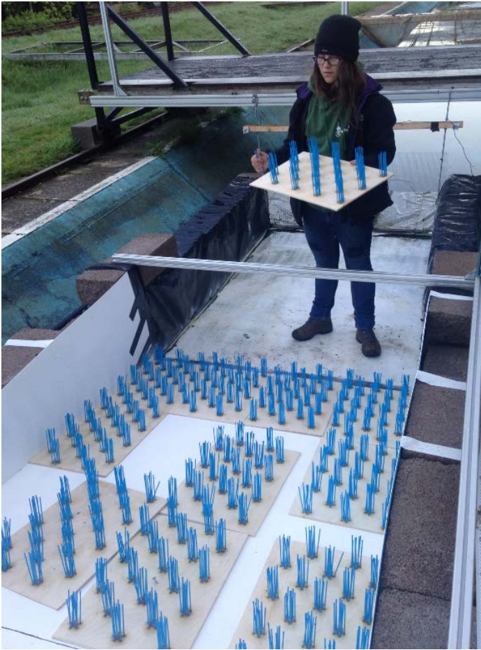
Figure A.2.1 CBC installation on the downstream face of the Crump weir used during experimental trials.
