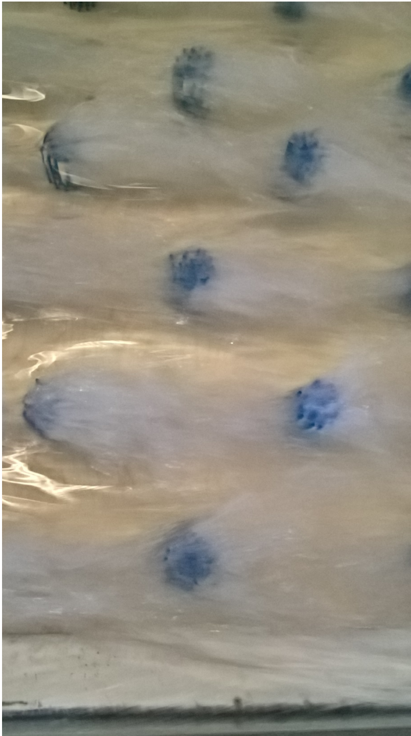
Figure A.7.7 A photograph of flow through a staggered array of clusters with flow overtopping the clusters in places dependent on placement within the array.
