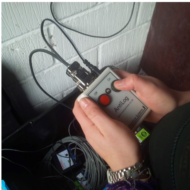
Figure A.3.5 Photograph of (a) the data logging setup and (b) equipment which was connected to the PIT loops installed on the weir
