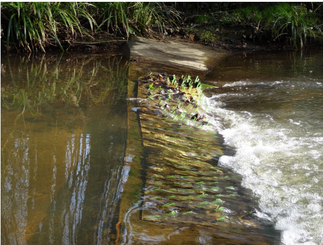
Figure A.1.5 Photograph of debris accumulation during field installation of the bristle boards (a) close up and (b) showing the whole installation.
