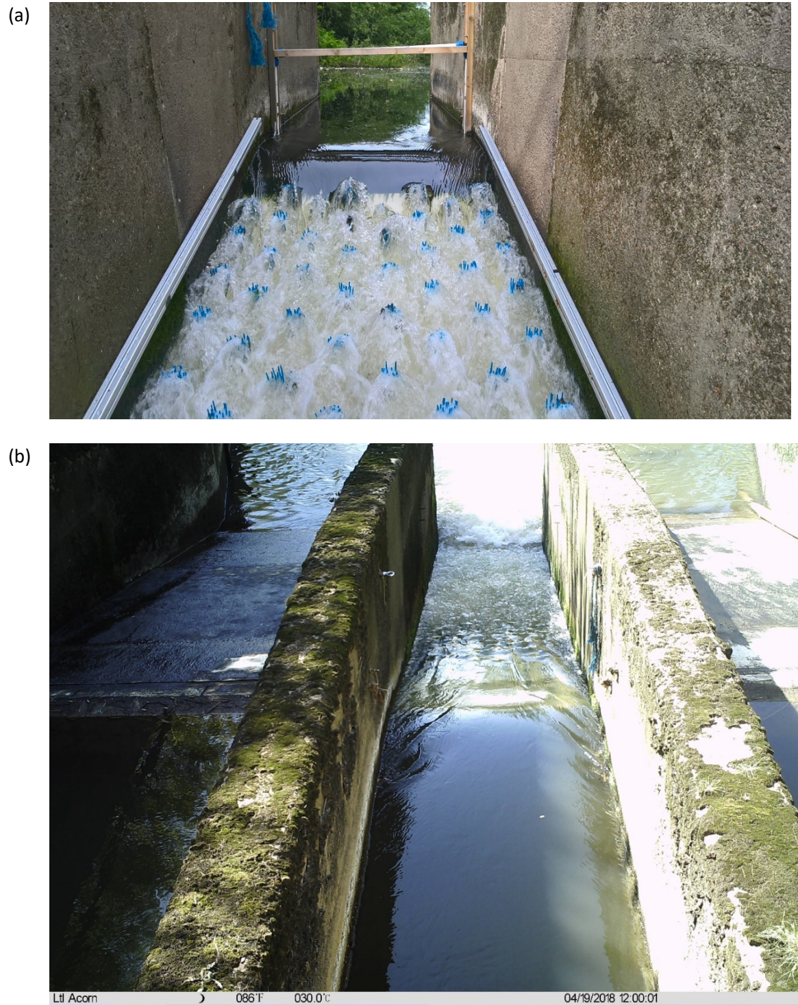
Figure A.3.3 Flow through the CBCs looking (a) upstream when the clusters were unsubmerged and (b) downstream when the clusters were only just submerged.
