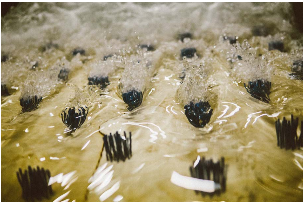
Figure A.7.11 Photograph of the water surface profile looking downstream with clusters only just submerged on the upstream end of the CBC array, progressively getting shallower.
