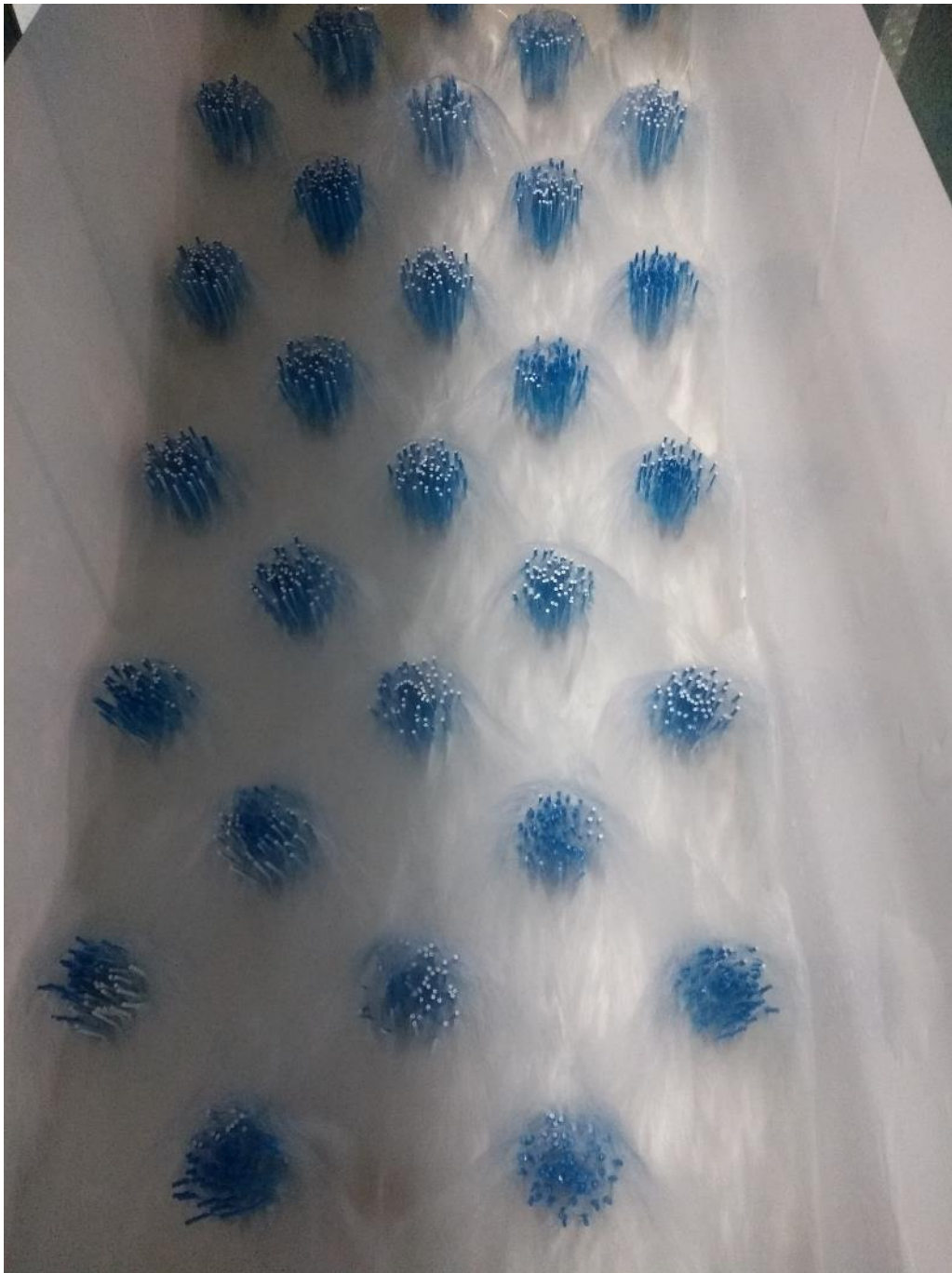
Figure A.6.1 Photograph from above with water running through a staggered array of clusters with 0.1 m diagonal spacing and 0.07 m diameter clusters.
