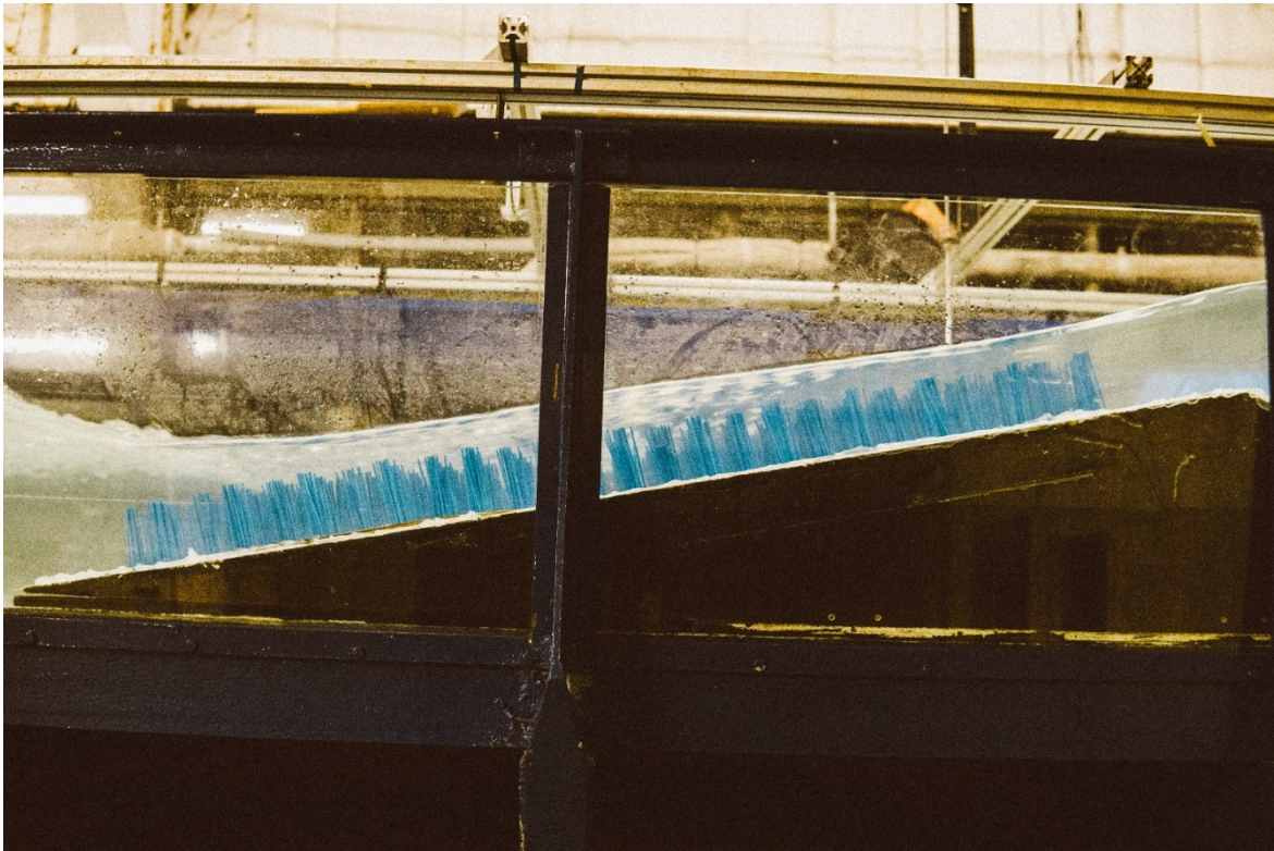
Figure A.7.9 Section view of the CBCs on the weir face showing the water surface profile under submerged conditions.
