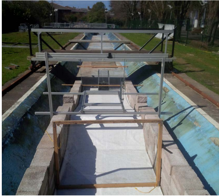
Figure 5.1 Photograph of the experimental setup showing the blocks used to create the rectangular channel within the flume, fish screens indicating the upper and lower extents of the experimental setup, the weir placed between these screens and the frame created using item bars to hold the camera recording fish movements. The photograph was taken looking downstream before the setup was complete.
