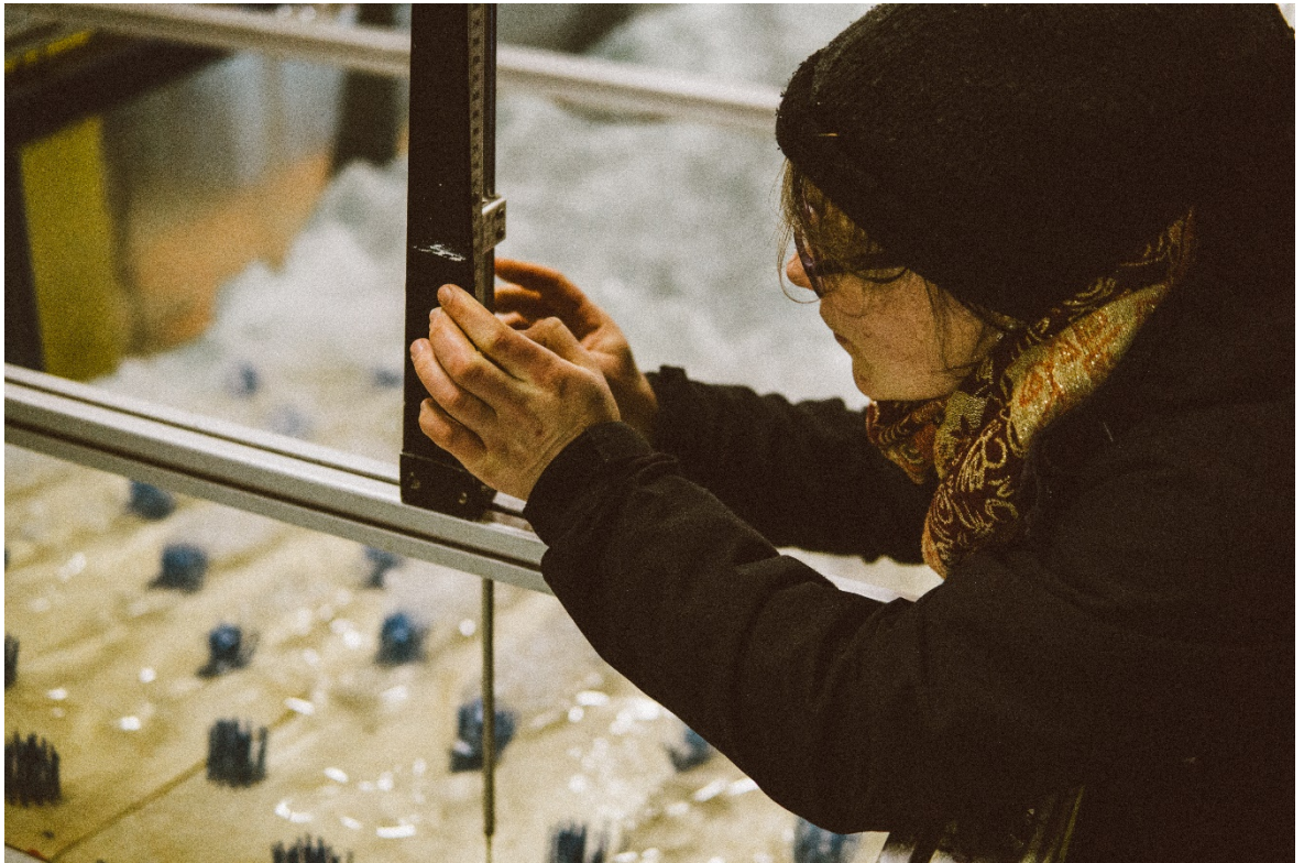
Figure A.7.2 Undertaking point gauge measurements upstream of the CBC array.
