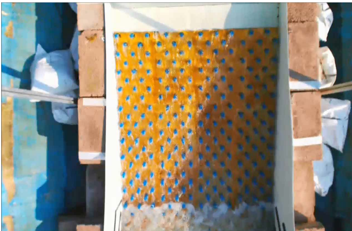
Figure A.2.3 View from above of the CBCs mounted onto the weir with water flowing from top to bottom of the photograph.
