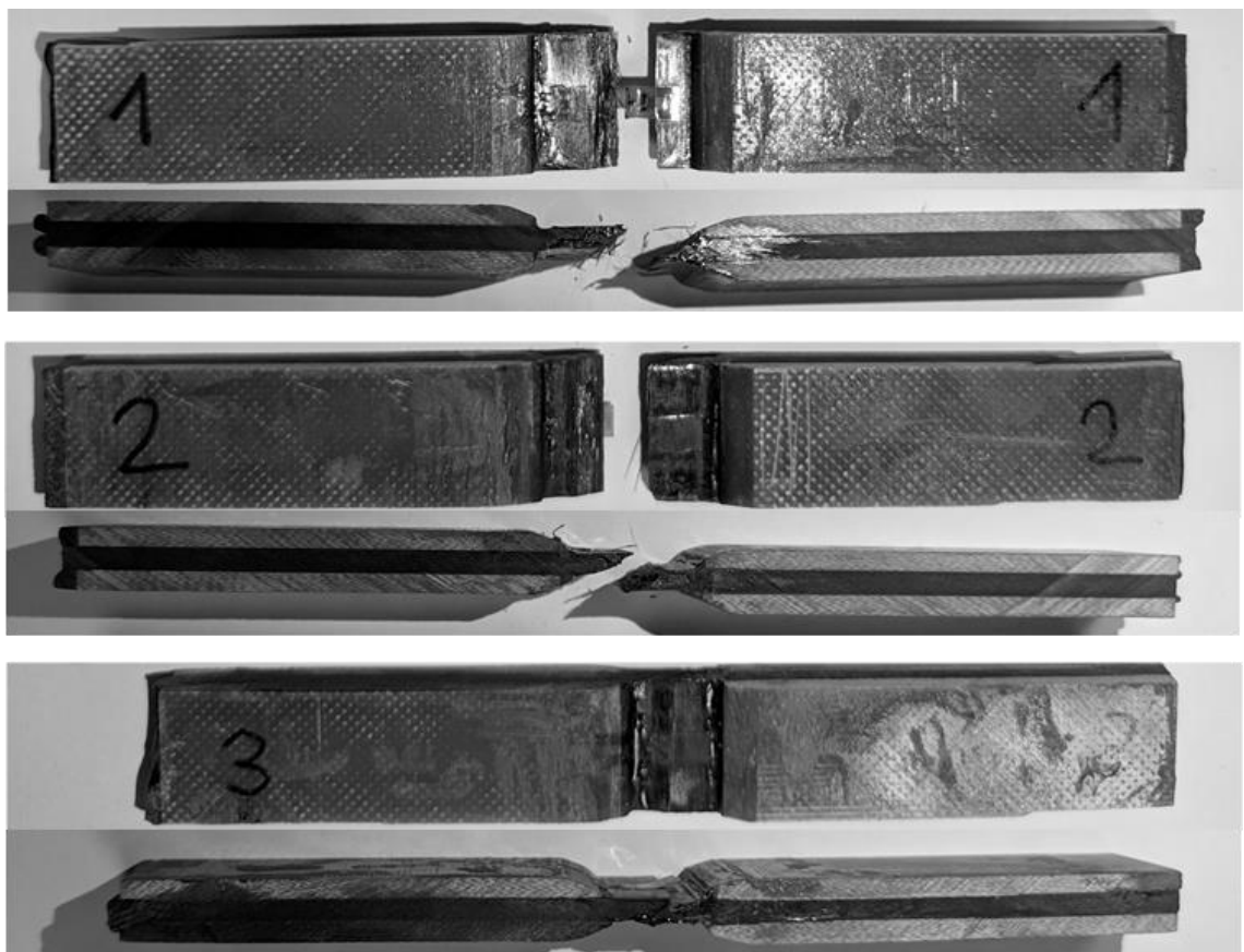
Figure C.18, Failed transverse compression specimens.
