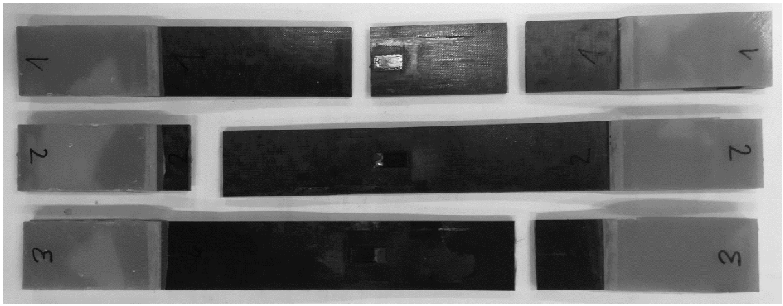
Figure C.5, Failed specimens showing transverse matrix cracks in the gauge area.
