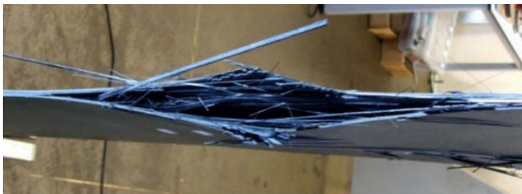
Figure 2.17, Example of a uniaxial tensile specimen that failed with excessive delamination [108].
