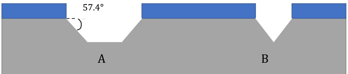
Figure A.22 Sidewall profile of Silicon etched in KOH
