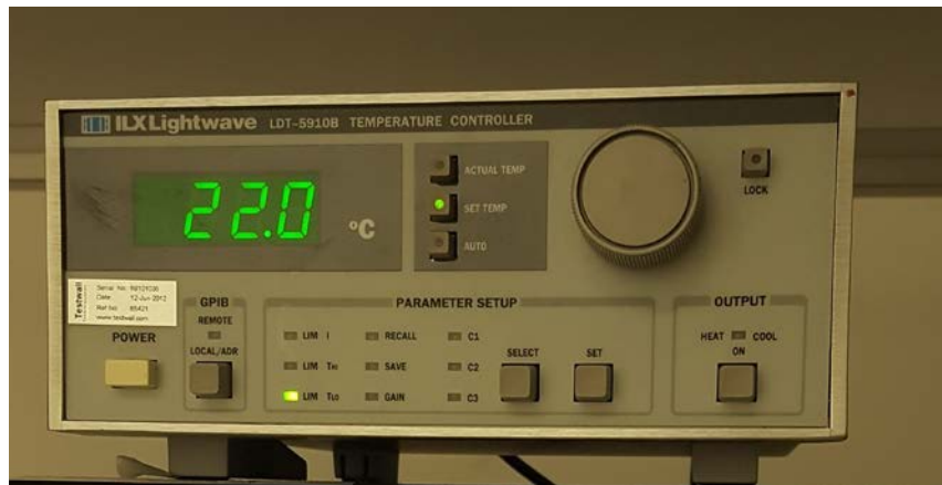
Figure 5.2 Photograph of the Newport Temperature Controller used for accurate optical measurements
