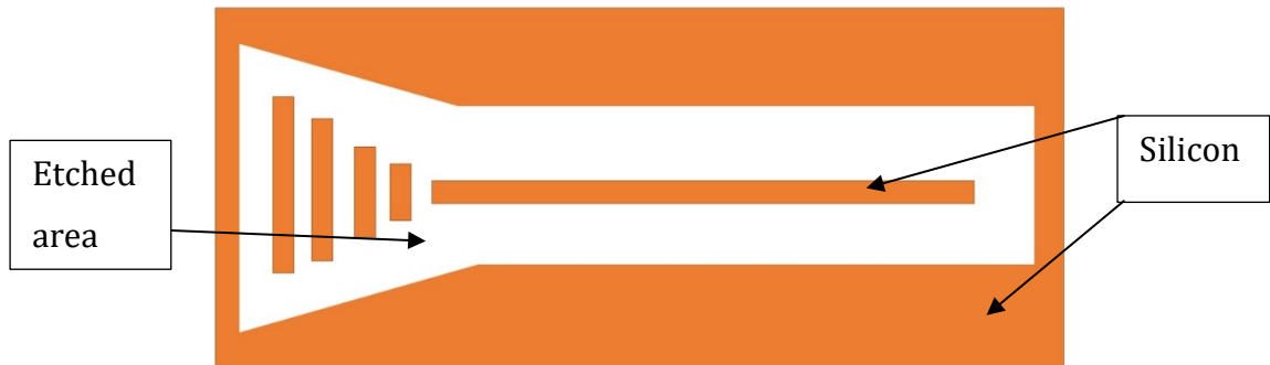
Figure 6.3 Diagram showing the e-beam etch outline
