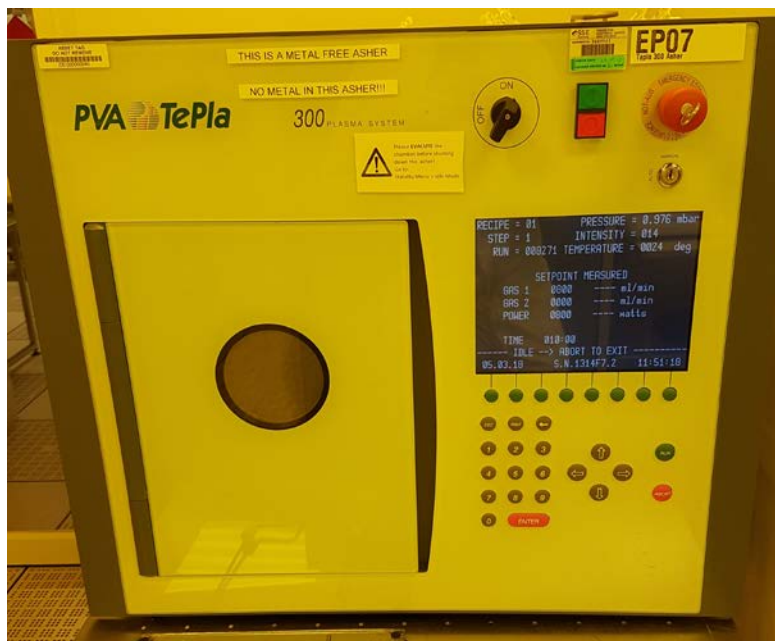
Figure A.12 Image of PVA Tepla 300 Plasma Asher in the SNC
