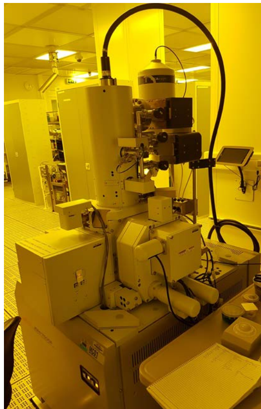
Figure A.33 Image of a JEOL JSM-7500F SEM used in the SNC
