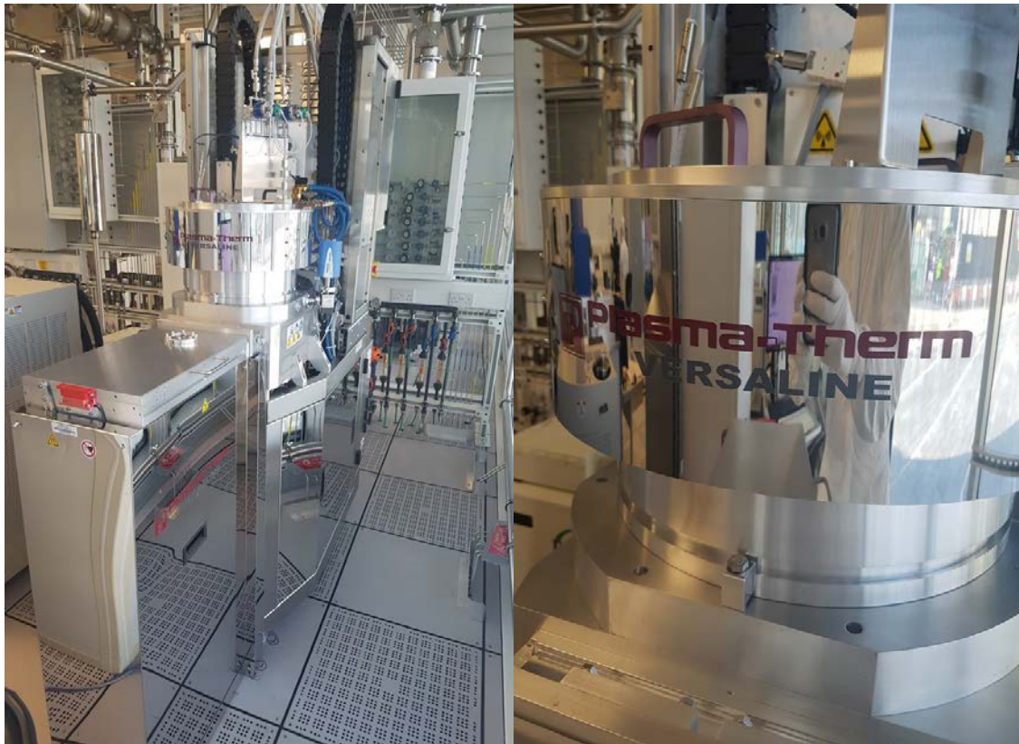
Figure A.19 Plasma-Therm Versaline DRIE
