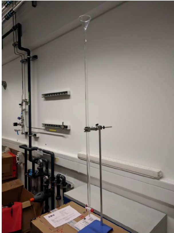
Figure 8.3 Image showing a method to separate different silica spheres
