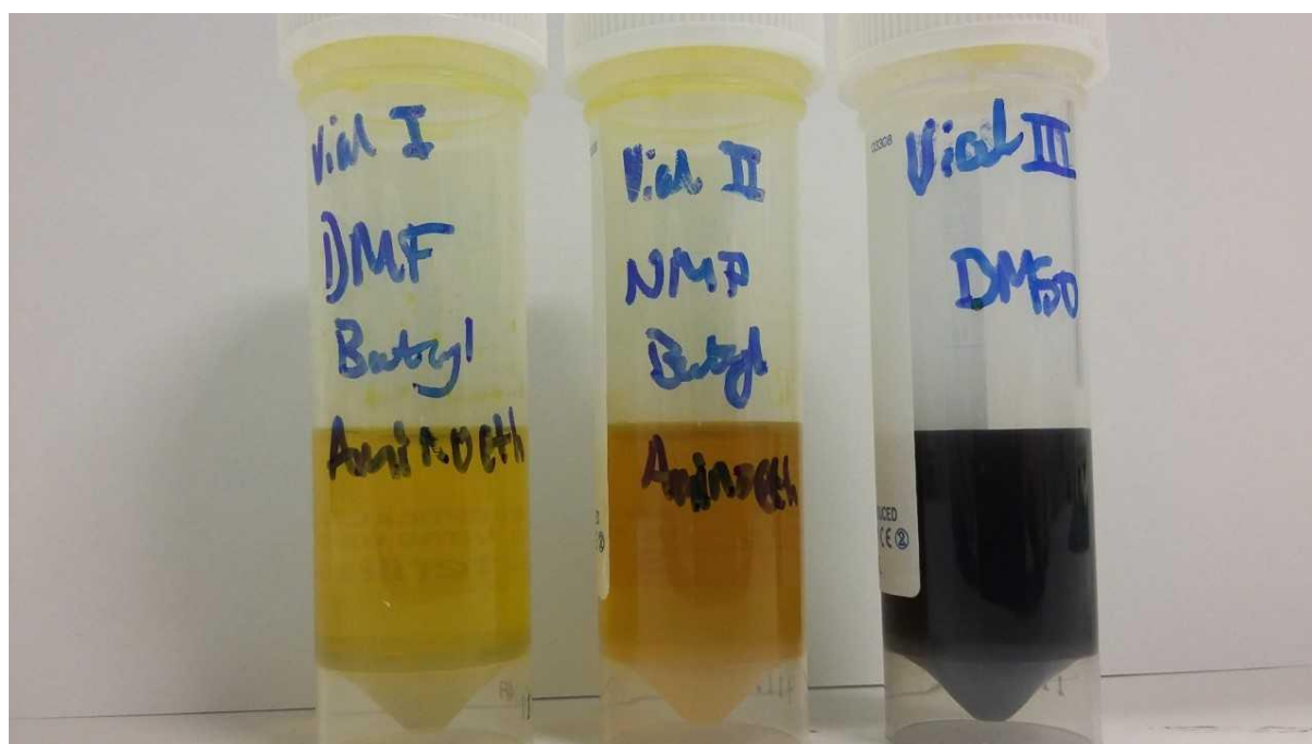
Figure 5.4: Images of the precursor solution in three host solvent solutions of DMF/Aminoethanol/Butylamine, NMP/Aminoethanol/butylamine and DMSO. Each has the same wt% at 1%.
