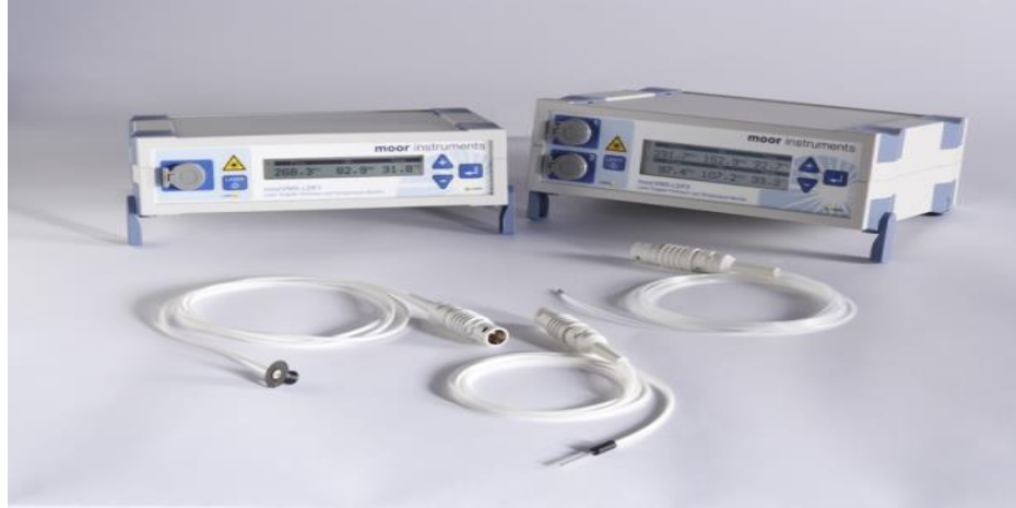
Figure 2.12 The combined blood flux and tissue oxygen monitor. Reproduced with kind permission from Moor Instruments Ltd.
