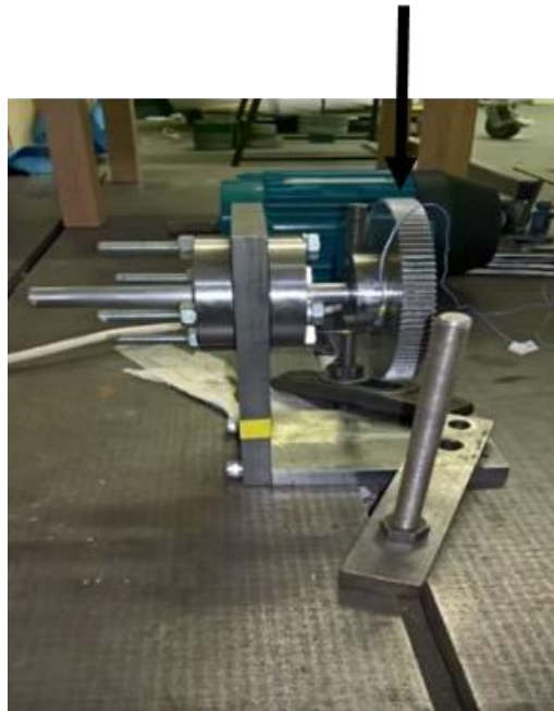
Figure 4-9 Set-up to determine sun gear bearing stiffness.
