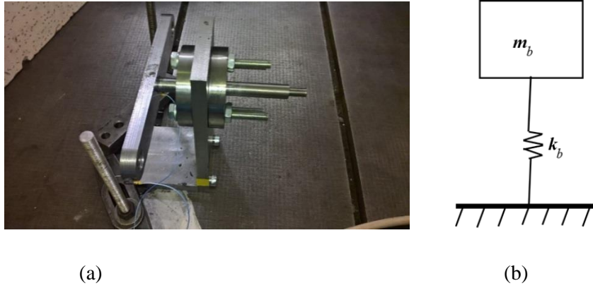
Figure 4-7 Set-up to determine carrier bearing stiffness using the (a) experimental and (b) analytical models.
