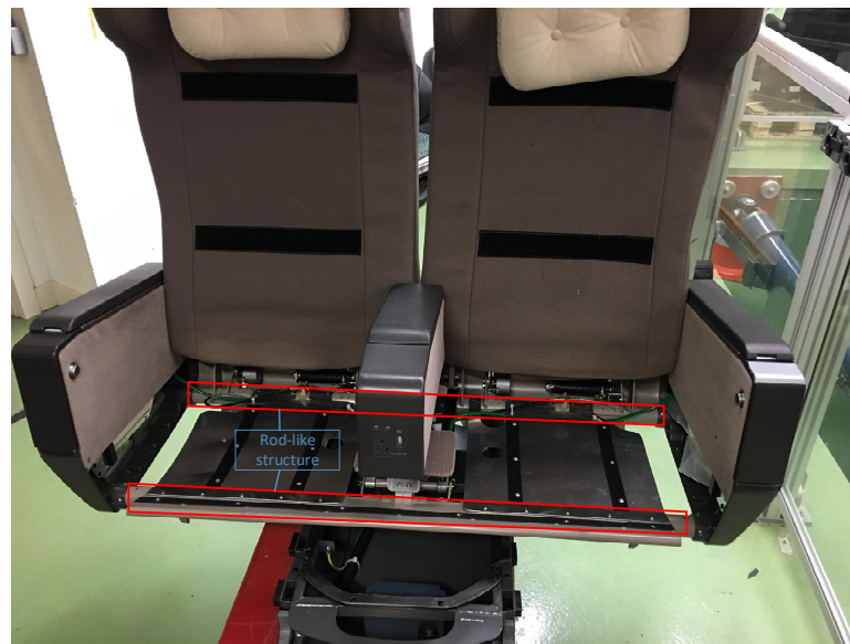
Fig. C-4 The internal structure of the train seat
