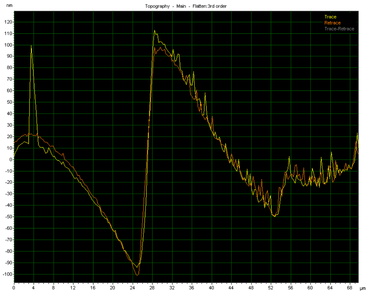
Figure 97: Trace-retrace plot of the sample number 9539 of the Au-Ni alloy system showing the film thickness.
