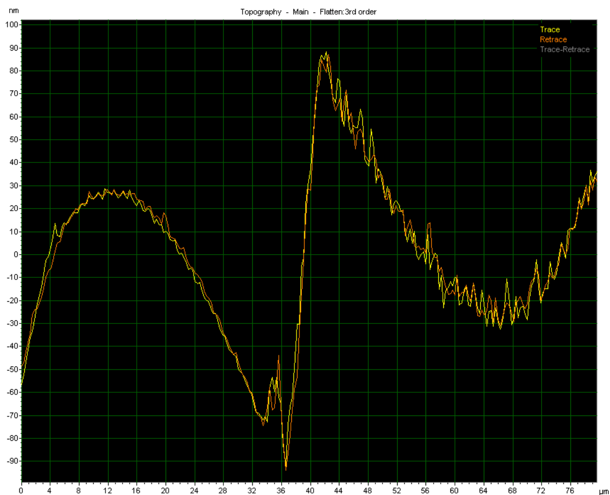
Figure 95: Trace-retrace plot of the sample number 9336 of the Au-Pt alloy system showing the film thickness.
