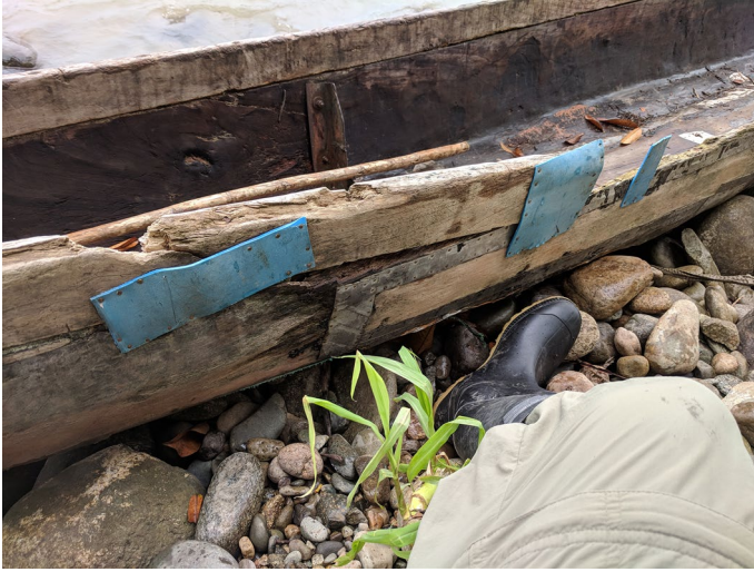
Fig. 4 Patches cut from plastic food barrels on an extended logboat, Rio Napo, Ecuador. (B. Holtzman)
