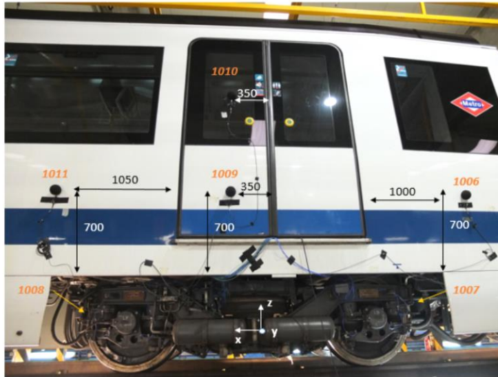
Figure 4.25. Field measurements to measure sound distribution on the train outside surface.
