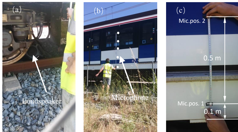
Figure 4.23. Measurements of sound pressure on a stationary train. (a) Loudspeaker location, (b) microphone positions, (c) separation of microphones. Photos provided by Polytechnic University of Valencia.
