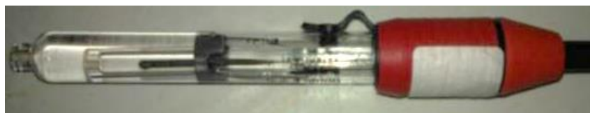
Fig. 3-11 Ag/AgCl reference electrode.
