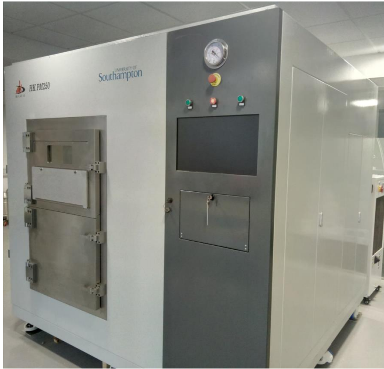
Fig. 3-5 HK PM 250 MM SLM machine developed at the University of Southampton.
