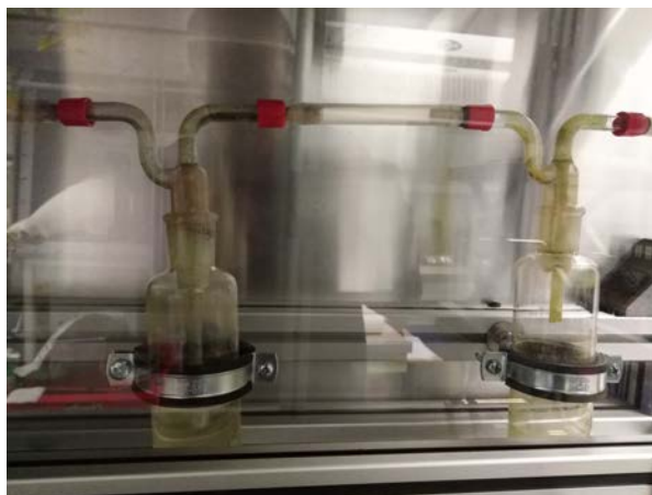
FIGURE 5.5: Glass vessels to filter any volatile particle from the melt before the extraction
