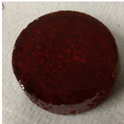
FIGURE 5.14: GLS-Se glass billet using the GAZ 3 crucibles and 30 g of raw materials
