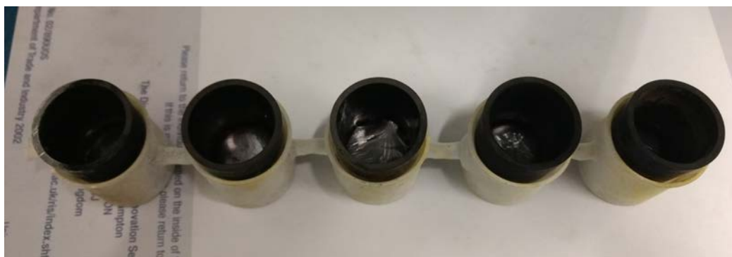
FIGURE 5.11: GLS-Se glass samples, after a successful melt quenching
