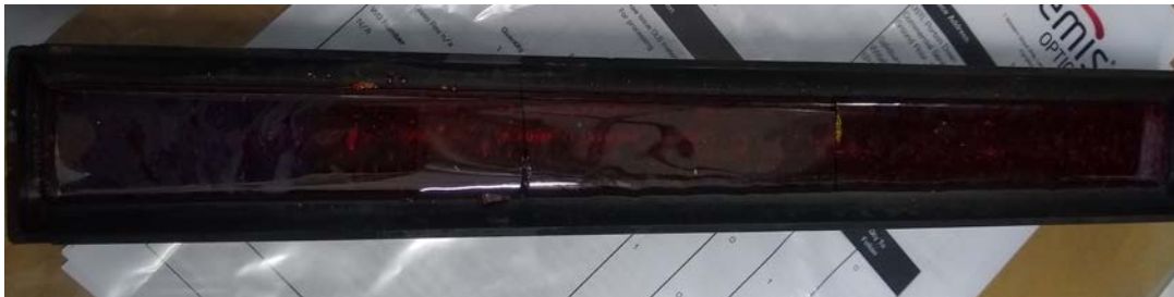
FIGURE 5.16: GLS-Se glass ingot for billets remelt
