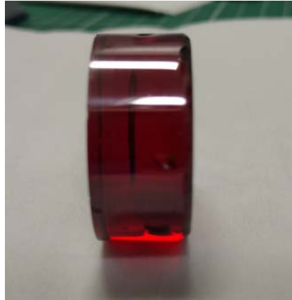
FIGURE 5.27: Billet cylindrical surfaces can be polished for different thicknesses
