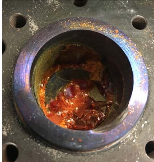
FIGURE 6.9: Example of crushed glass, as the lid and piston were positioned incorrectly
