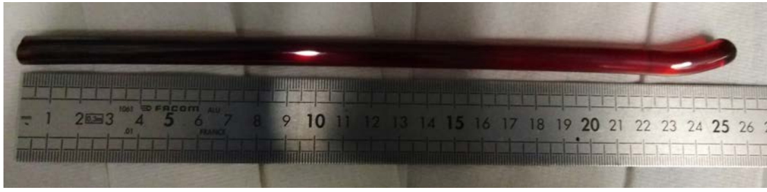
FIGURE 6.25: GLS-Se extruded rod without crystals and with a maximum length of 26 cm
