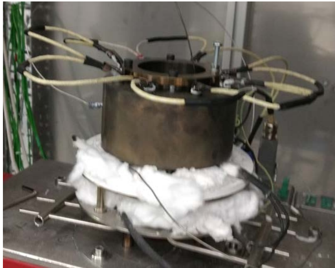
FIGURE 6.7: Partially assembled extrusion apparatus showing the main heating element before the ceramic shield is placed
