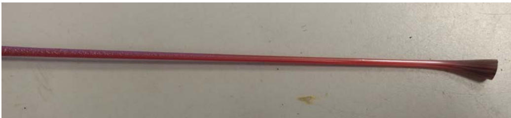
FIGURE 7.15: GLS-Se cane after cracking due to a high tension as the temperature was too low for fibre drawing
