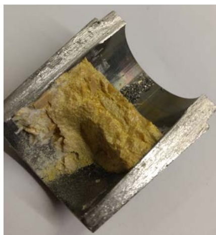
FIGURE 6.12: Ceramized GLS sample after a failed extrusion attempt
