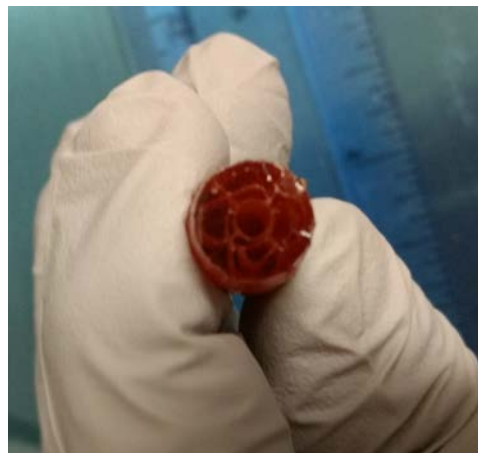
FIGURE 7.12: Transparent glass in the inside, surface crystallized
