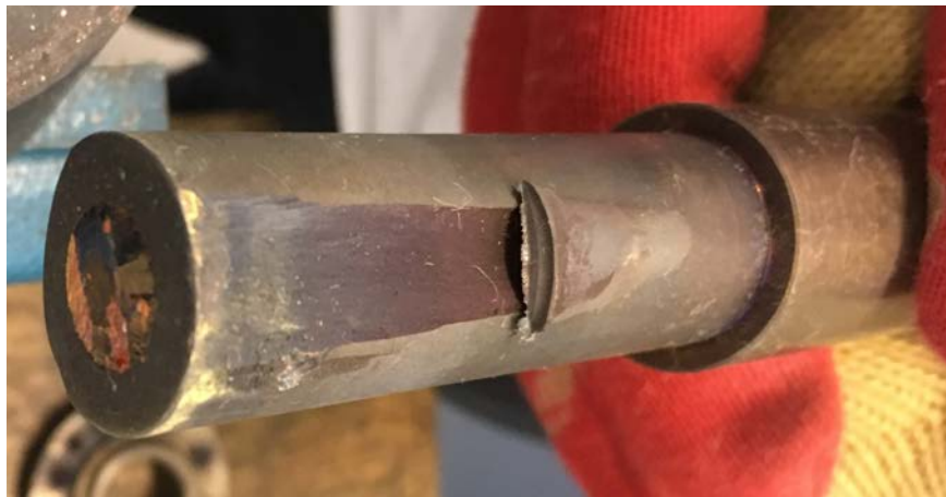
FIGURE 6.3: Damaged piston after mispositioning it in the extrusion apparatus
