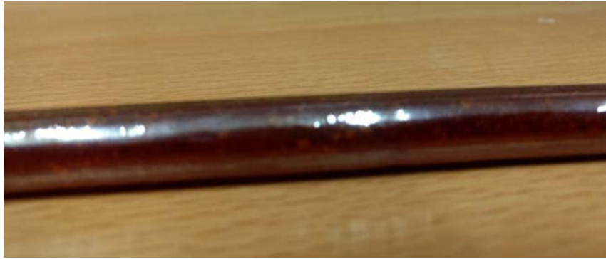
FIGURE 6.15: Extruded preform partially crystallized as billets were unpolished
