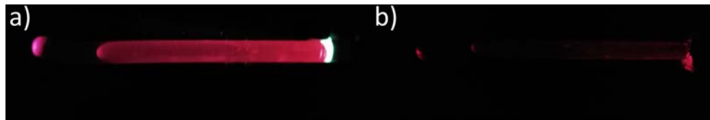
FIGURE 6.28: Structured preforms under a white light source showing the scattering in the core-clad interface, where a) shows a heavily scattering preform and b) scattering was suppressed
