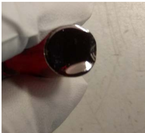
FIGURE 7.16: GLS-Se glass rod showing an amorphous phase and transparency proving that the furnace does not affect directly the glass in the temperature is low and it is not exposed to heat for a long time
