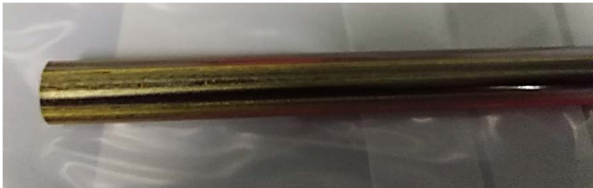
FIGURE 6.22: Extruded rod with surface defects caused by partially crystallized billets
