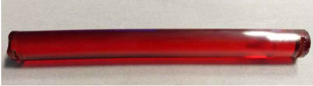
FIGURE 7.1: Extruded glass rod of 10cm after being cut to fit the drawing furnace
