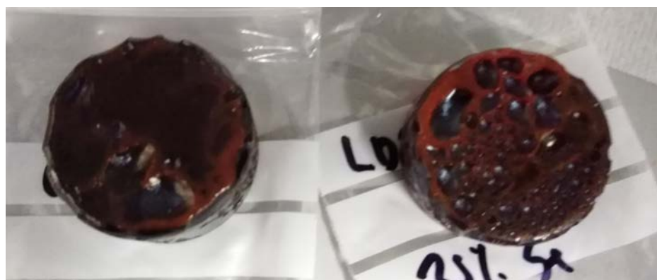
FIGURE 6.21: Billets for extrusion not completely transparent, just the bottom part of them presented this anomaly
