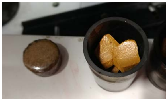
FIGURE 5.9: Crystallized samples, not usable for further processes
