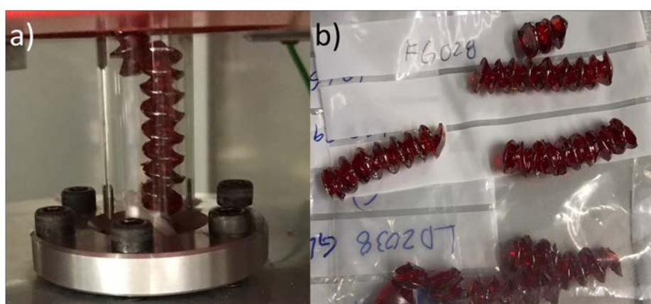
FIGURE 6.20: Twisted extrusion due to a malfunctioning in the heating elements, where a) is the extruded glass inside the protection tube and b) samples of the failed extrusion
