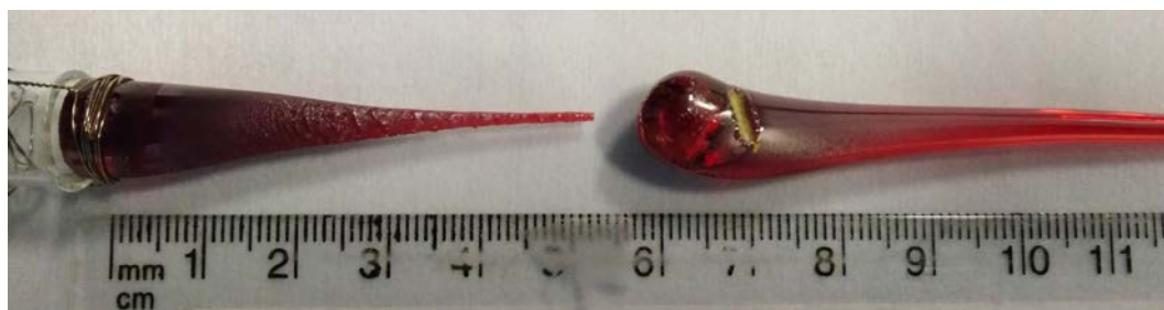
FIGURE 7.23: First and last part of the extruded rod after fibre drawing, where the neck presents some surface crystallization due to the time consumed in the whole process
