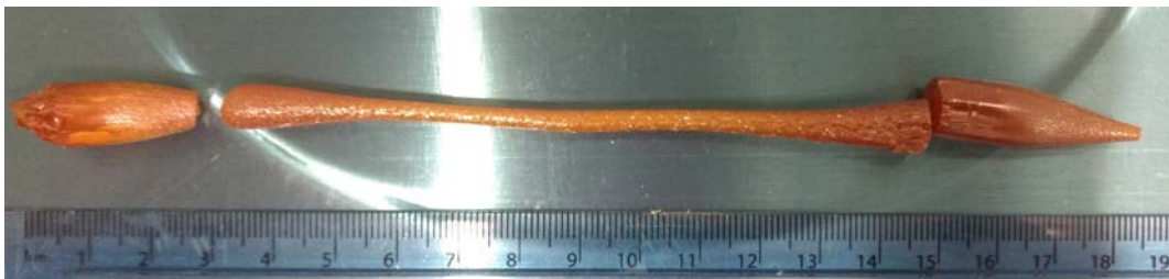
FIGURE 7.11: Unsuccessful GLS extruded drawing attempt
