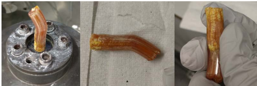
FIGURE 6.14: Extruded GLS sample, heavily crystallized as glass was crushed during extrusion and a wrong temperature was set
