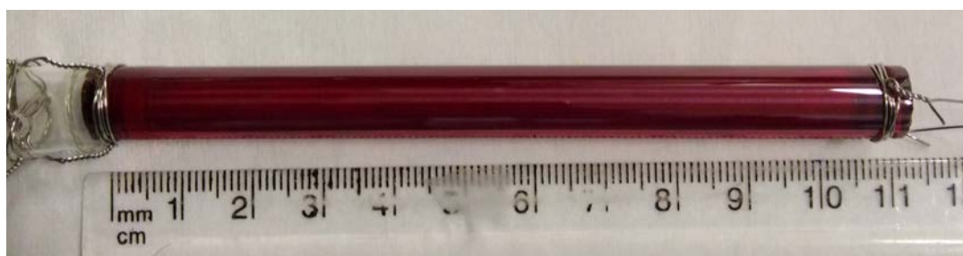
FIGURE 7.8: Extruded and polished rod of 11 cm ready to be set on the furnace, surface quality is clearly seen
