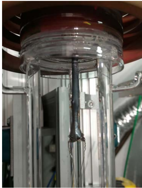
FIGURE 7.14: Glass rod coming out the furnace showing the necking and before any crystallization occurred
