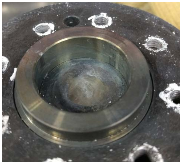
FIGURE 6.6: Billet container, showing a gap between the lid and the sleeve favouring the positioning of the piston
