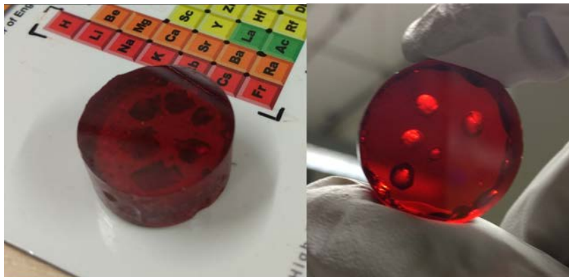
FIGURE 5.23: GLS-Se sample after optical finish ready for measurements. Note: the bubbles are only in the bottom part of the billets
