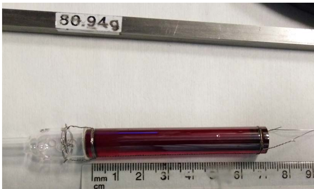
FIGURE 7.7: Extruded and polished rod attached to the silica holder and the 80 g weight
