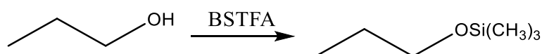
Figure 2.1. Derivatisation reaction used on Tetraselmis extracts to convert OH groups into silyl groups increasing response factor of polar compounds in GC-MS analysis.
