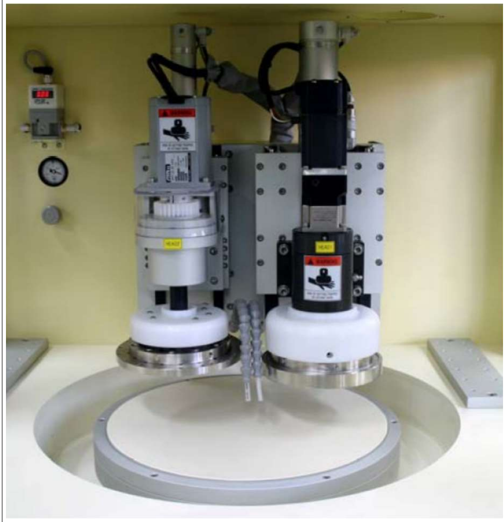
FIGURE 3.14: CMP tool showing the polishing table/platen with the white polishing pad, the conditioning head on the left, the polishing head/wafer holder on the right, and the central tubes for dispensing slurry and DI water to the rotating pad.
