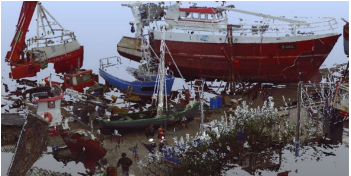
Figure 4-12 Three-dimensional registered point cloud from the six scans in Figure 4-10 (Pat Tanner)
