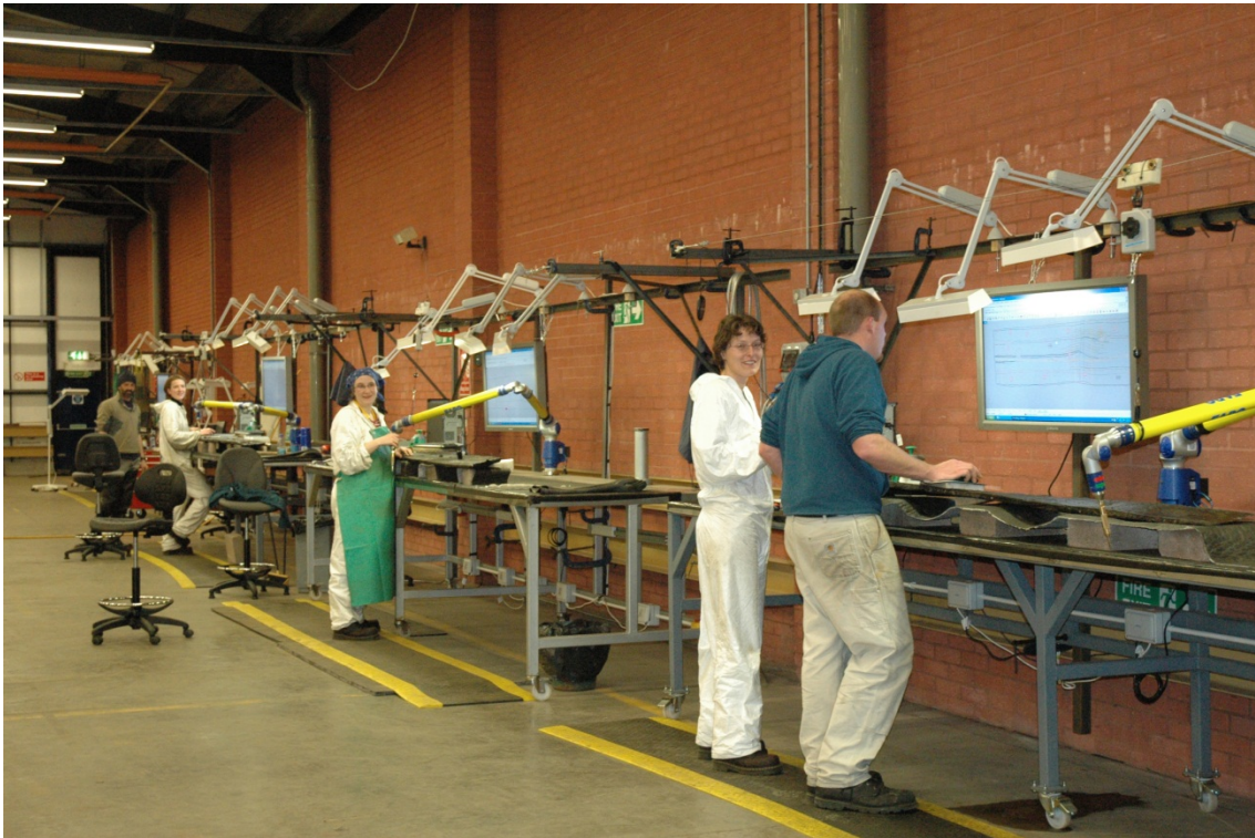
Figure 4-19 Four identical contact digitiser work stations were created to efficiently record the large assemblage. (Photo: Newport Museums and Heritage Service)
