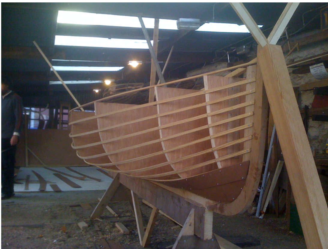
Figure 8-3 Temporary moulds and lightweight fairing battens to ensure a fair hull form, note the lofting floor in the background with planking being developed (Pat Tanner)
