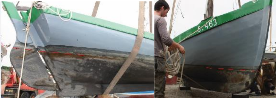
Figure 6-12 Digital photographs clearly showing the flotation waterline
