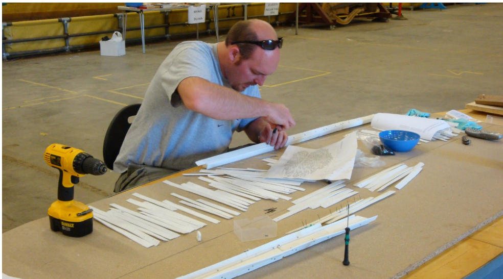
Figure 7-16 Toby Jones assembling model strakes. The sequence was visually documented using time-lapse photography (Newport Museums and Heritage Service)
