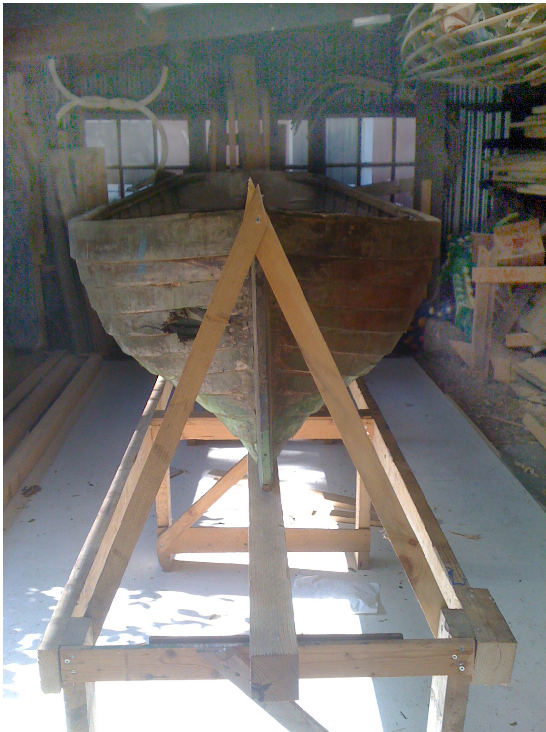
Figure 8-2 The original vessel positioned on the strongback (framework) and re-orientated level (Pat Tanner)
