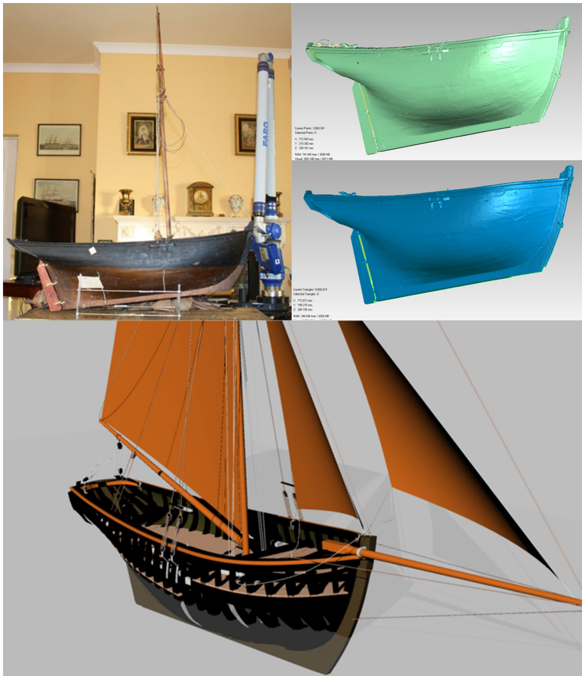
Figure 1-4 Kinsale Hooker scale model, 3D point cloud, surface mesh model and full-size digital reconstruction (Pat Tanner)
