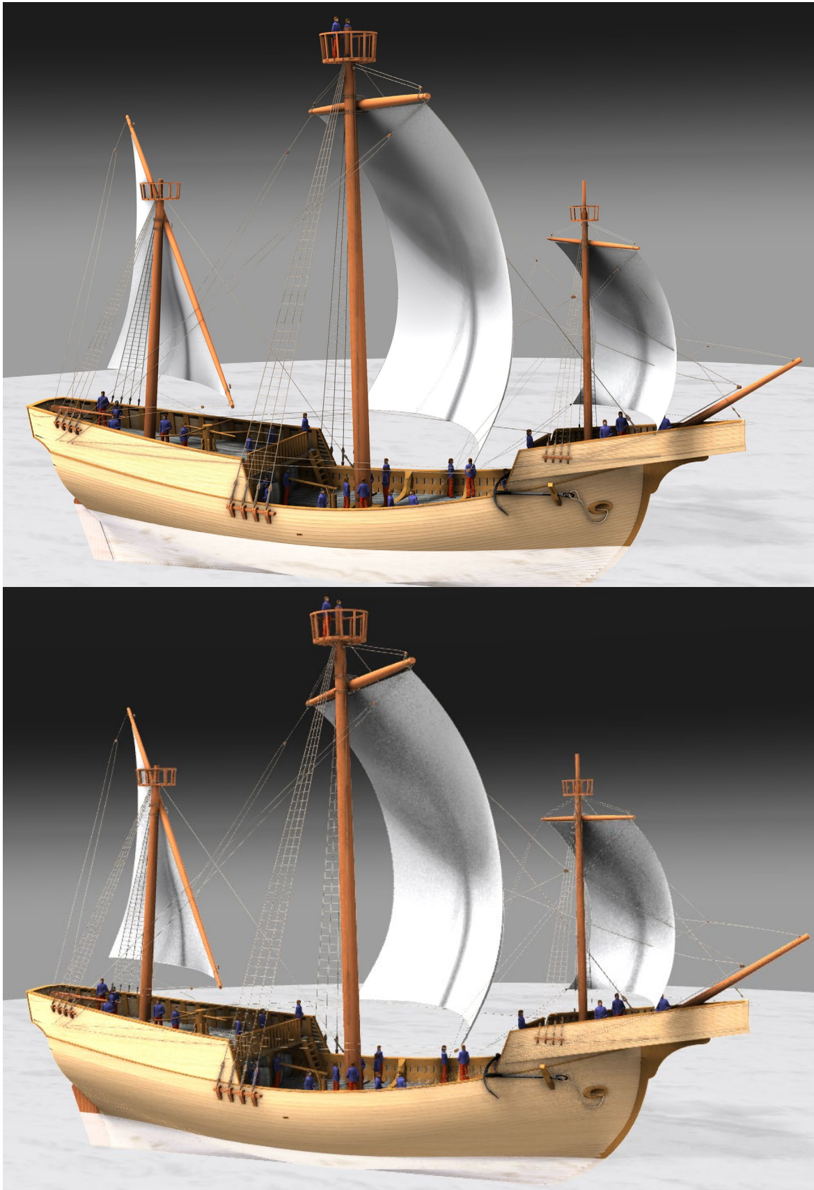
Figure 9-2 Newport Medieval ship – comparison between fully loaded flotation (top) and without cargo (bottom) (Pat Tanner)
