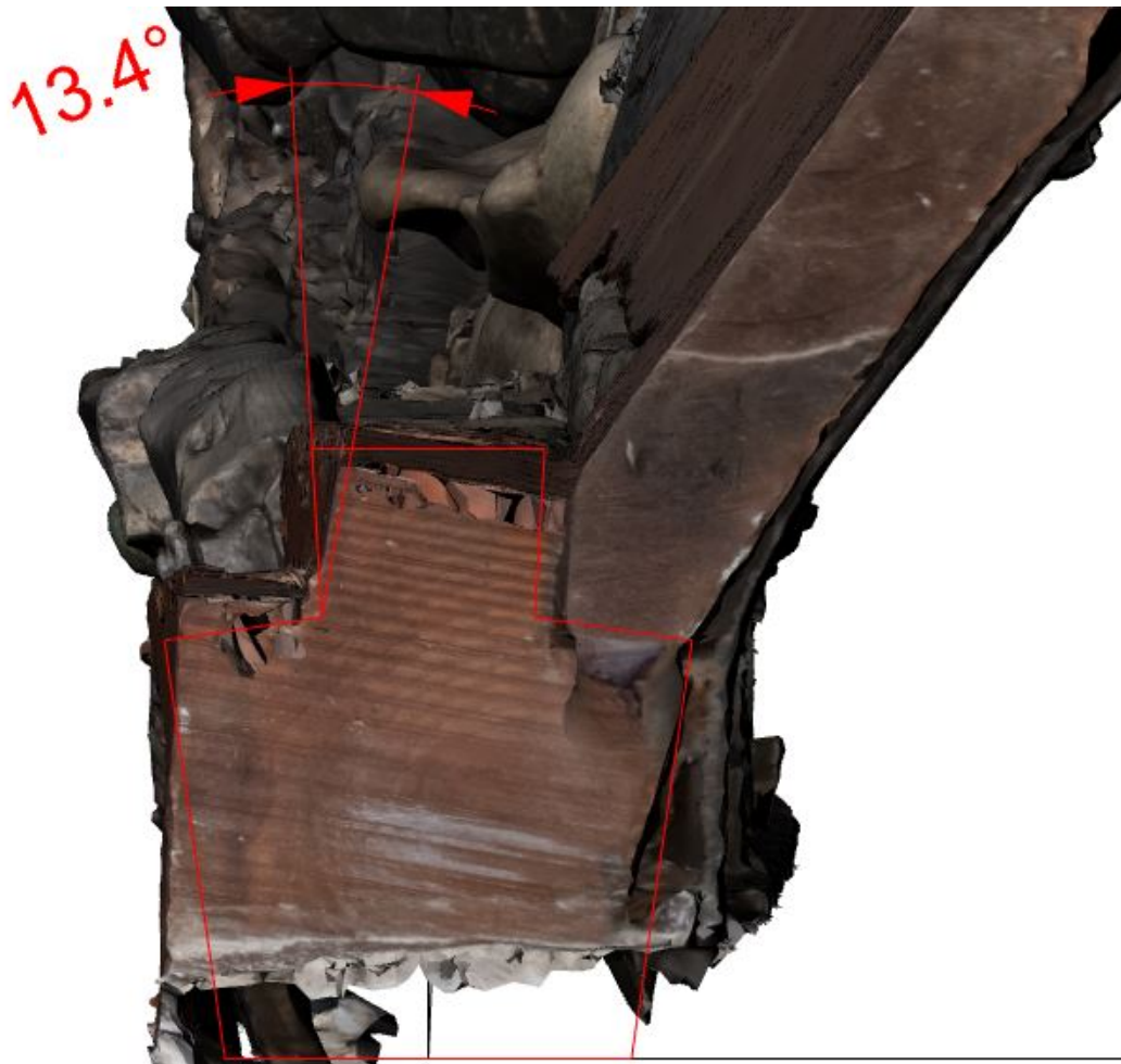
Figure 7-37 Cross section at the extant extremity of the remains showing the significant degree of twist (Pat Tanner)
