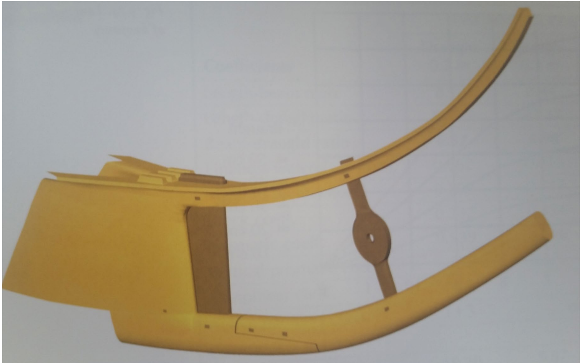
Figure 2-49 NURBs surfaces applied to the recorded data (after F. Hocker in Crumlin-Pedersen and Trakadas 2003)
