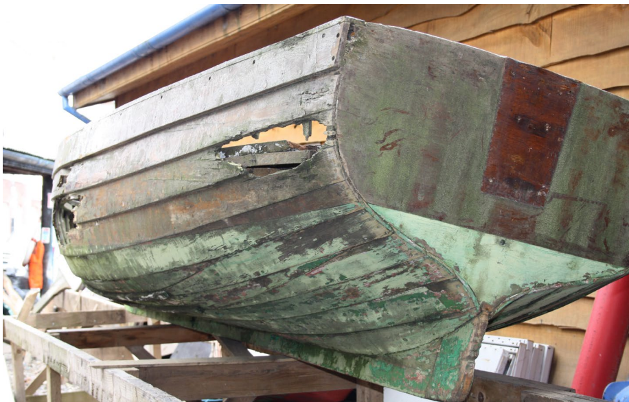
Figure 8-1 The original damaged and distorted vessel lying at an arbitrary angle (Pat Tanner)
