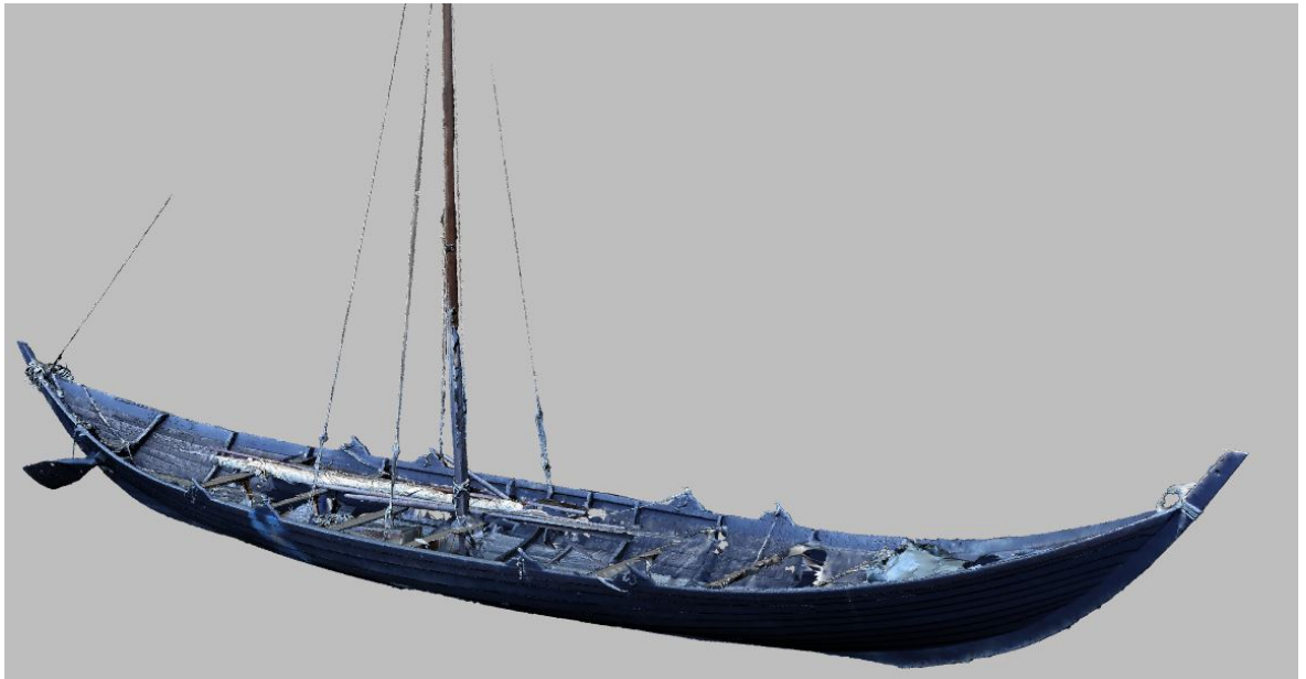
Figure 5-2 3D laser scan completed in 2018 of Sae Wylfing the half-scale Sutton Hoo replica (Pat Tanner)
