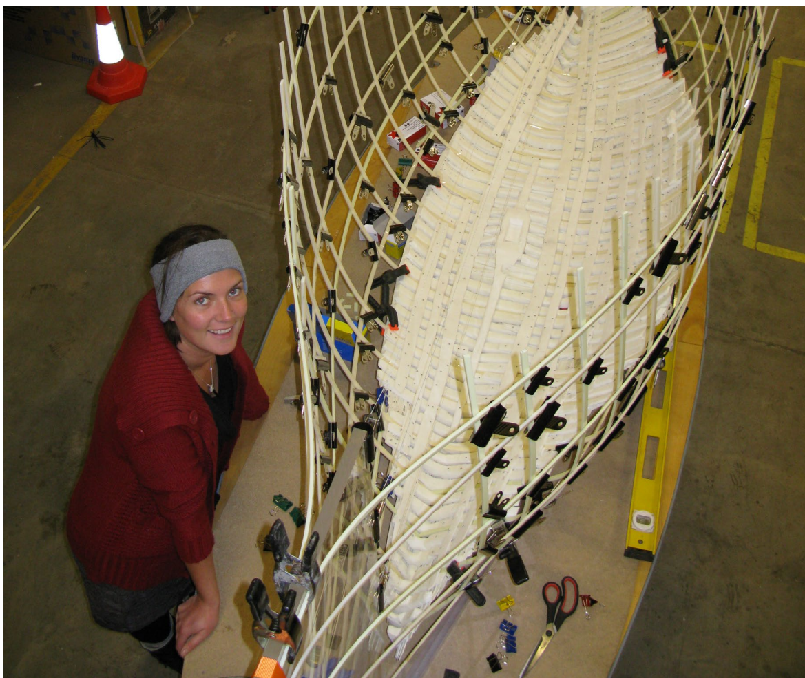
Figure 8-14 Physical scale model with fairing battens ‘forced’ into a double-ended hull form (Newport Museums and Heritage Service).
