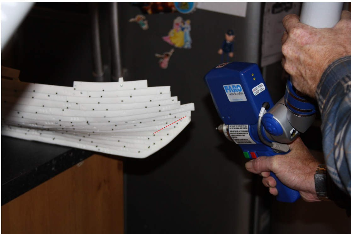
Plate 2: 3D Laser scanning the reconstructed scale model (H. Schweitzer)
