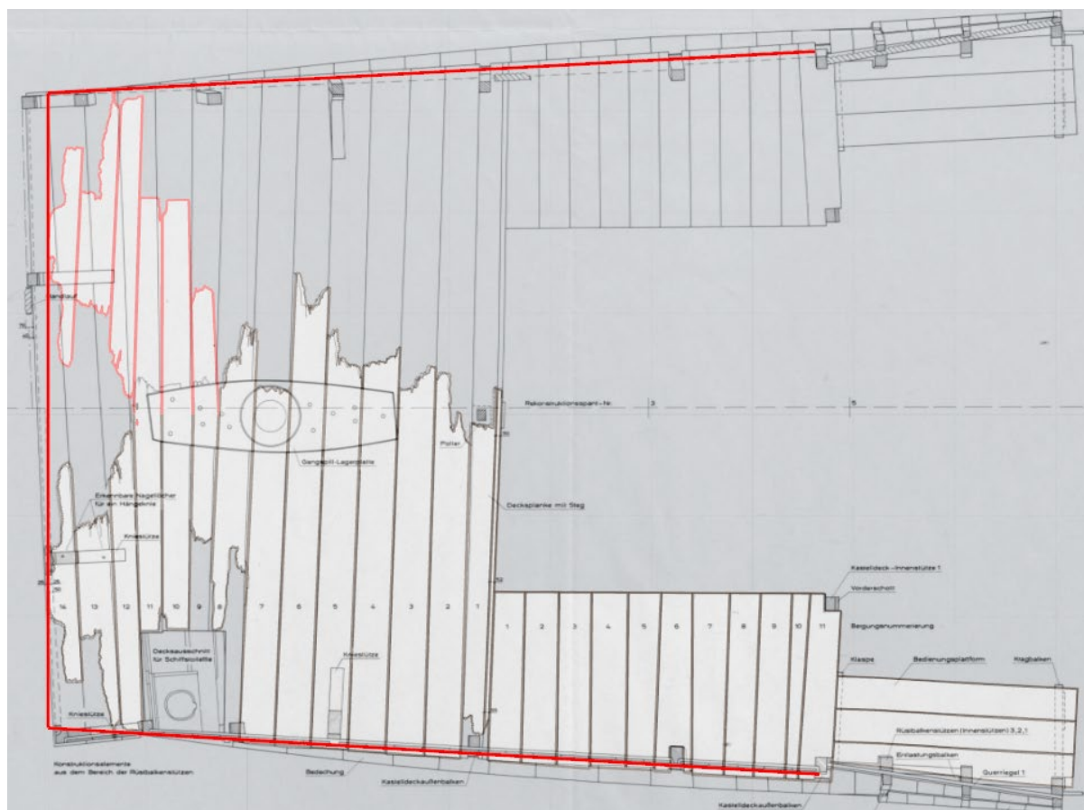
Figure 74 mirroring the deck planks to create an alternative stern castle end
