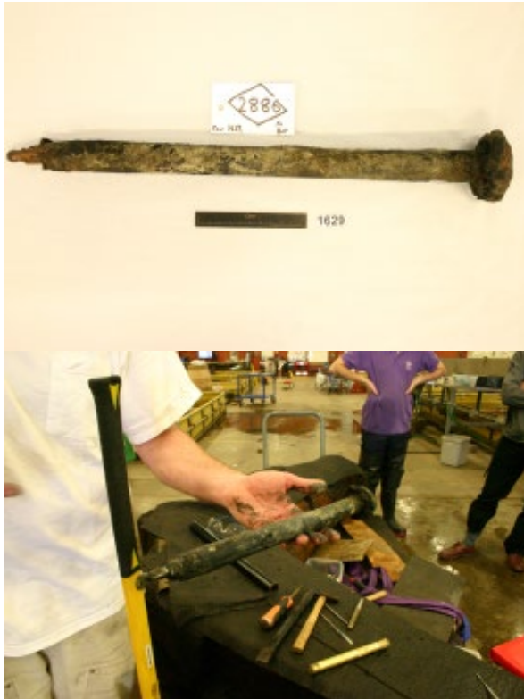
Figure 46 Iron forelock bolts associated with Knee CT1629 (Newport Museums and Heritage Service)
