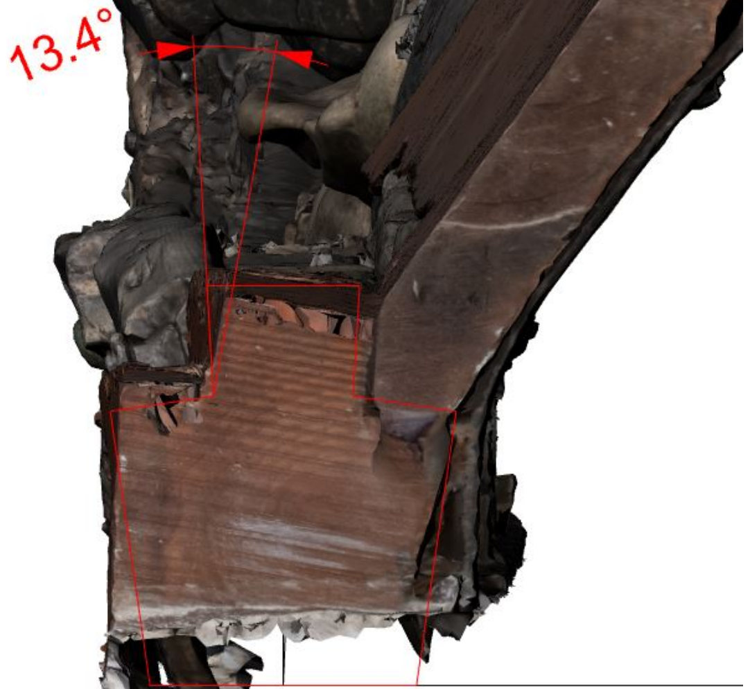
Figure 13 Keel twist towards midship extremity
