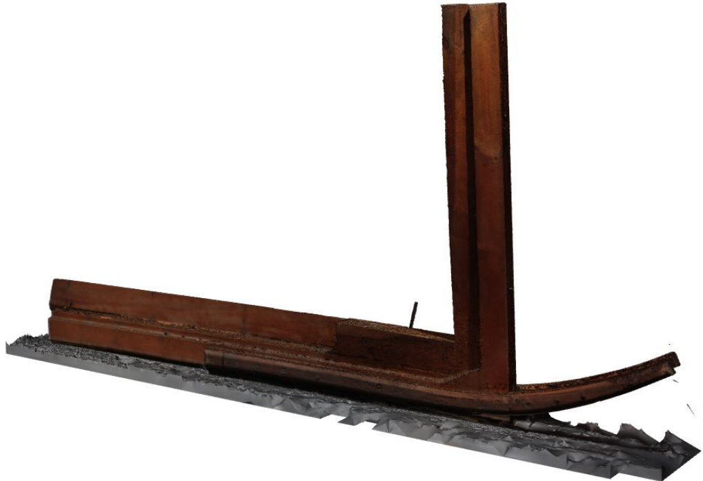
Figure 10 High resolution 'Sister ship' stem model imported into Rhino
