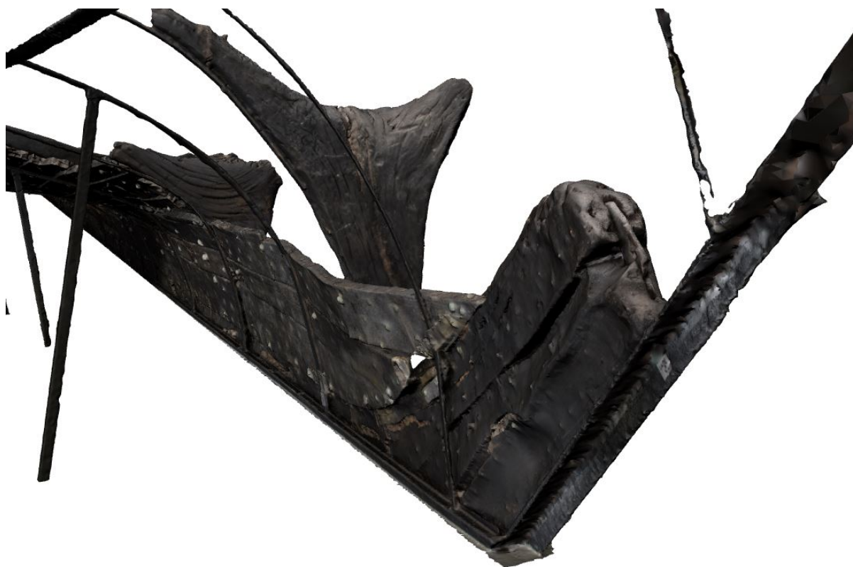
Figure 37 View of the displaced aft-most recovered frame and distorted port strakes
