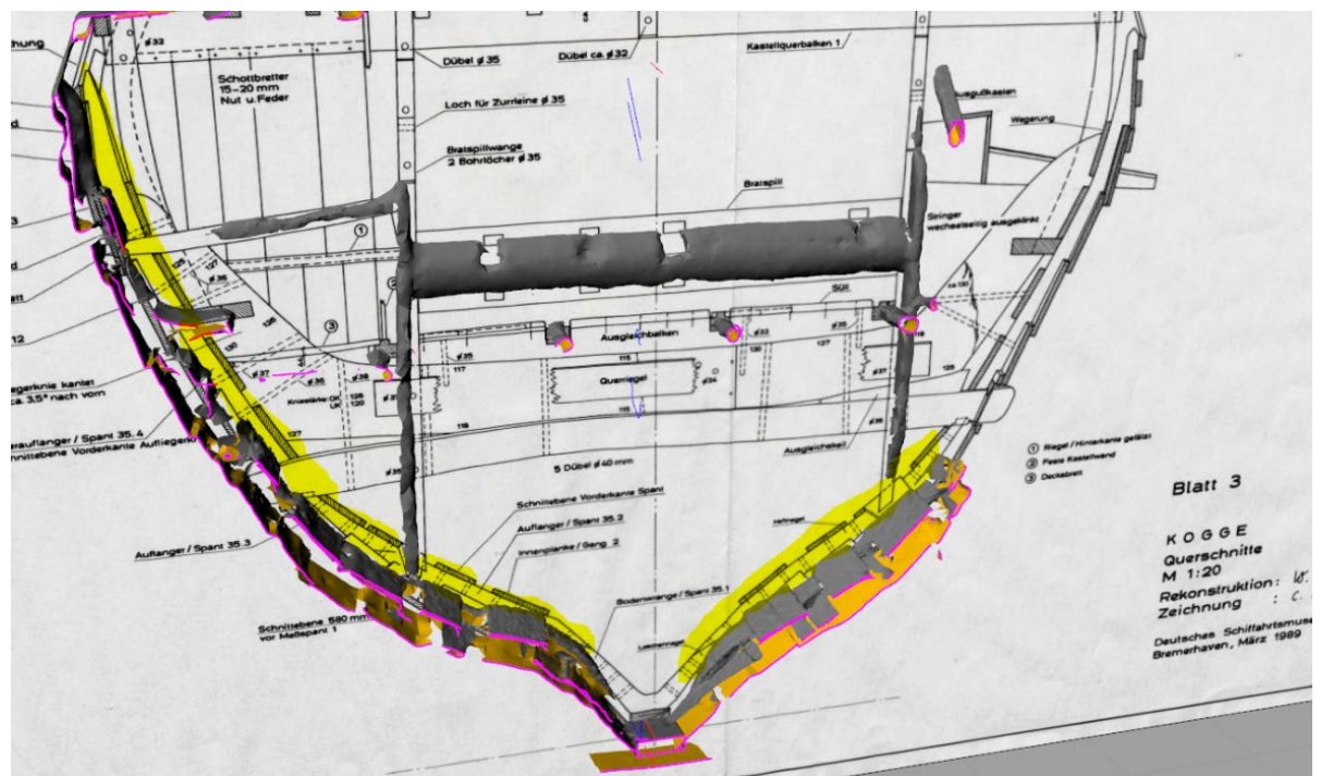
Figure 33 Drawing of Section at Frame 35 positioned over 2011 3D scan
