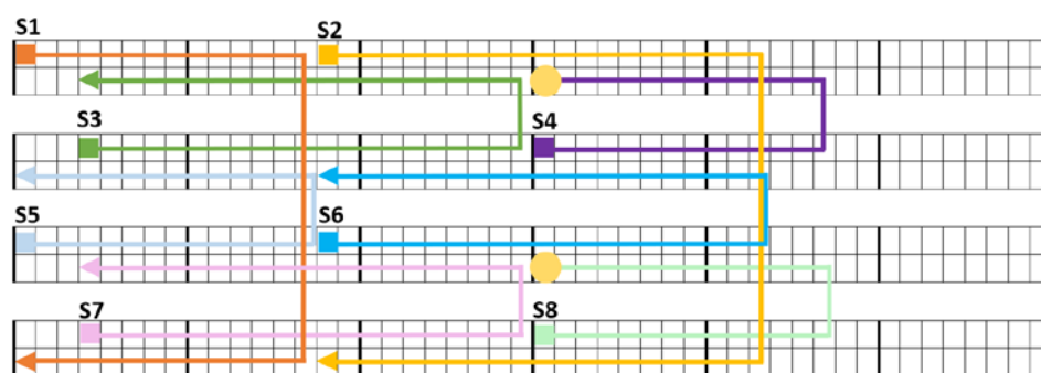
Figure 36 A schematic of the small nanopore in a form used by Cadnano, each squared grid represents a helical domain with each individual square representing a nucleotide. The solid filled squares represent the 5' terminus of the DNA and the solid triangles, the 3' terminus. DNA strands and crossovers are clearly shown by the different coloured arrows.
