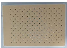
Figure 87 LED Light device that was used for light treatments. The relevant 96- well plate was removed from the IncuCyte and placed in the laminar flow hood. The device was placed on top of the lid of the 96 well plate and wrapped in foil to avoid light leakage before being turned on to the highest setting.
