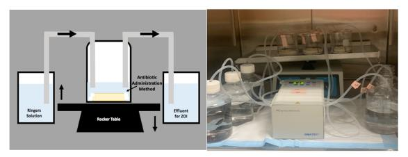
**Figure 7.** Schematic and real image of the in vitro draining knee reactor system. The system was placed onto a VSR-50 laboratory platform rocker at a frequency of 5 RPM. Ringers solution was pumped into and out of the reactor vessel at flow rates derived from post-operative surgical drainage rates.
