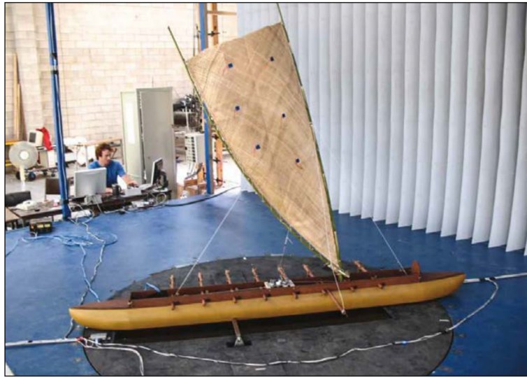
Figure 4.7: Model of an outrigger investigated in Irwin and Flay (2015). This is used as a proxy for the Outrigger or n'Drua design which succeeded the Tongiaki design. Note that the outrigger hull itself is missing from the model and would have been connected to the end of the wooden booms.
