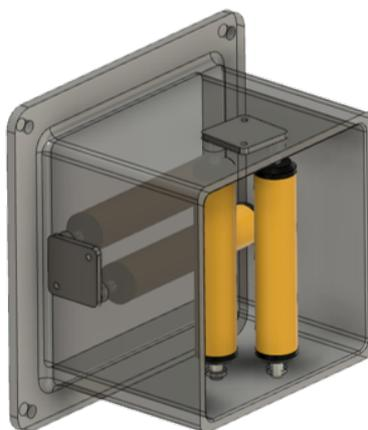
Figure 6.9: A 3D CAD drawing of the input roller box.
