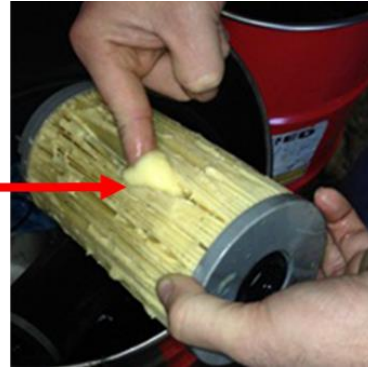
Figure 5-2 - Biodiesel type contamination on fuel filter, adapted from 253
