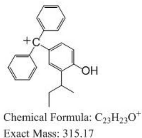
Figure 6-14 - EI fragmentation structures for ACCUTRACE™ S10 fuel marker
