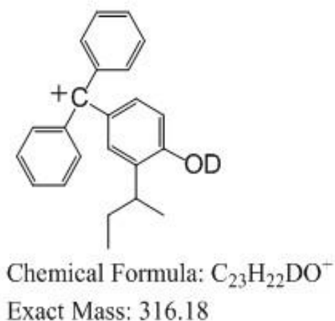
Figure 6-15 - EI fragmentation structures for ACCUTRACE™ S10- d_{21} internal standard
