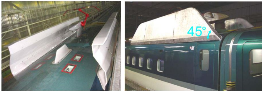
Figure 2.10: Z-shaped (left) and conventional (right) insulation plates studied by Kurita et al. [17].
